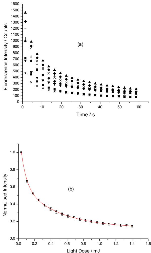
Fig. 2. mTHPC photobleaching recorded from a set of 10 cells (keratinocytes in 0.044 mM mTHPC for 3 hours) in the form of (a) fluorescence intensity as a function of time and (b) normalised fluorescence intensity as a function of light dose. The solid line represents an empirical bi-exponential fit to the mean data points. Laser power is 0.024 mW.
