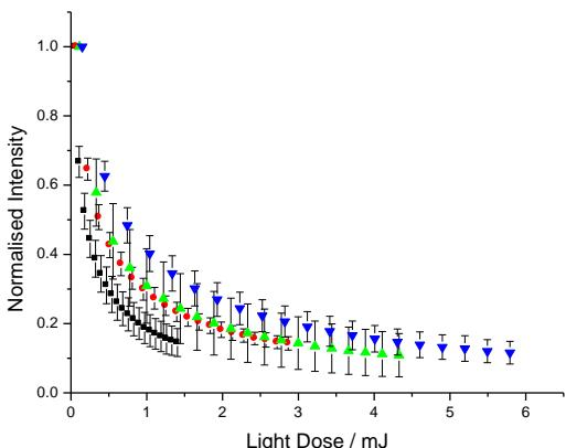
*Fig. 4.* Photobleaching plot of mTHPC showing the normalised averaged data points from sets of keratinocytes (in 0.044 mM mTHPC for 3 hours) exposed to different laser powers: 0.024 mW (■), 0.049 mW (▲), 0.074 mW (▼) and 0.099 mW (◆). Error bars are removed for clarity.
