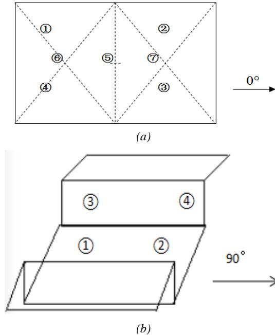
Fig.1 Pre-embedded positions of PFBG in composite materials (a) in the first and second series of experiments (b) in the third series of experiments
