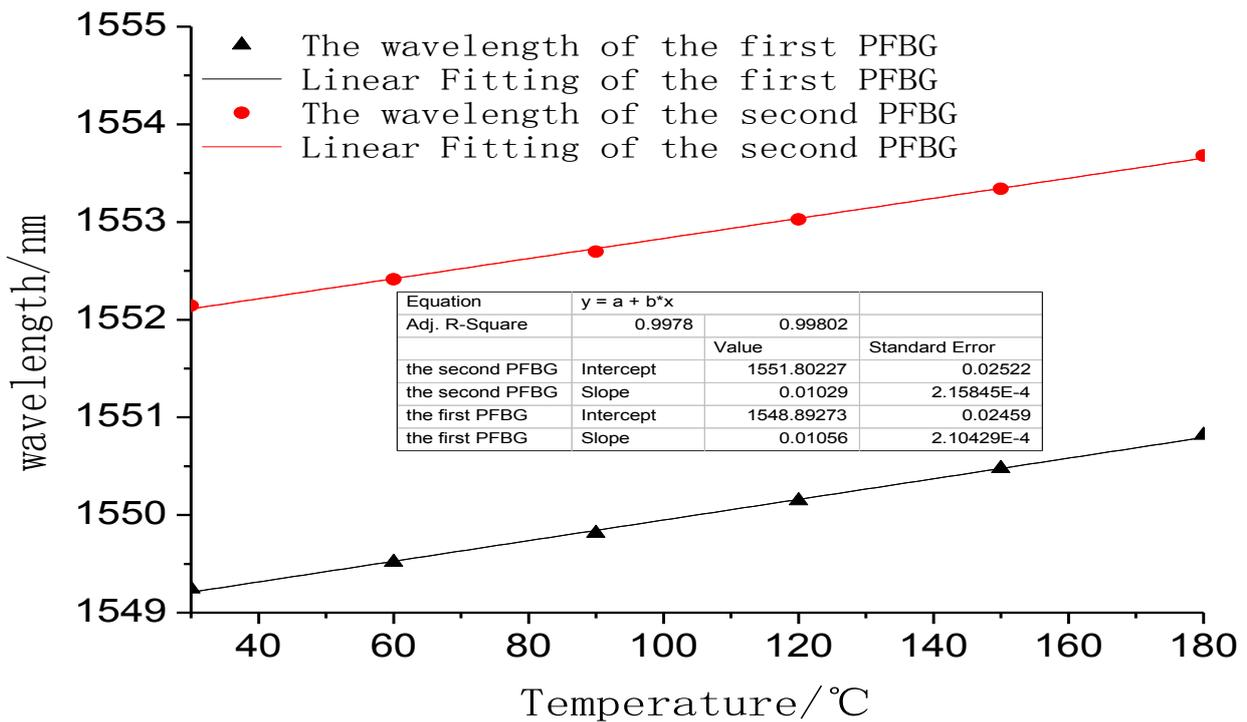
Fig. 3. Central wavelength measurements of PFBG
