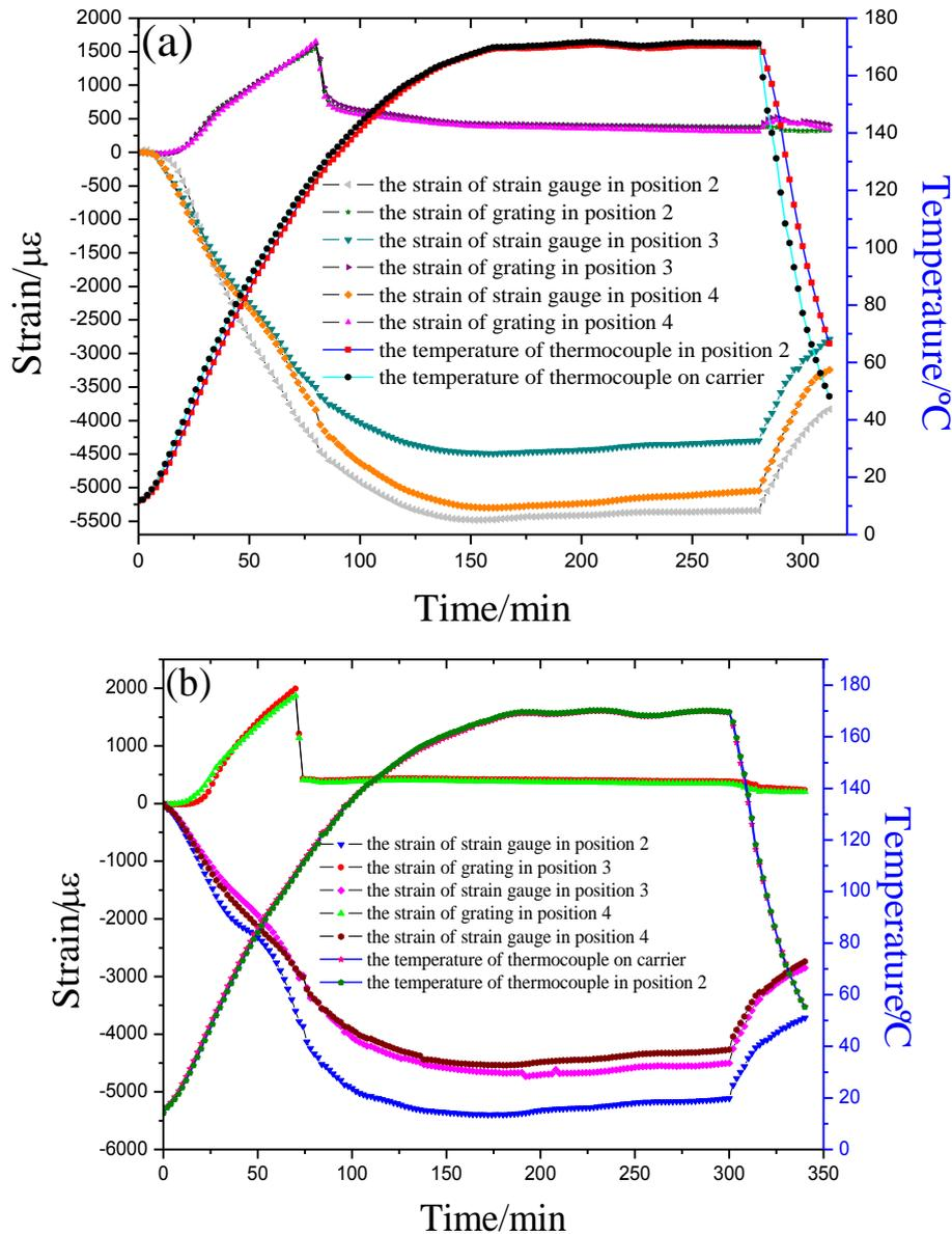
Fig. 5. The results of strain measurements (a) in the first series of experiments (b) in the second series of experiments (color online)
