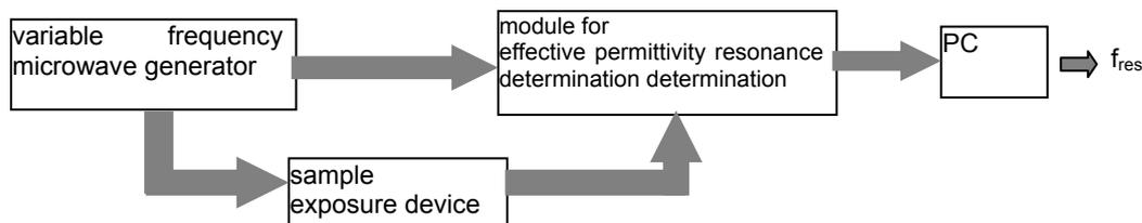
Fig. 1. Block diagram of the experimental setup for sample resonance determination.
