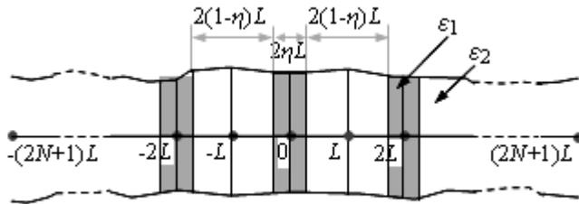
Fig. 2. Mixed stratified material, with alternative parallel layers, considered by Dukhin and Sihlov theory (after B. P. Scaife [8]).
