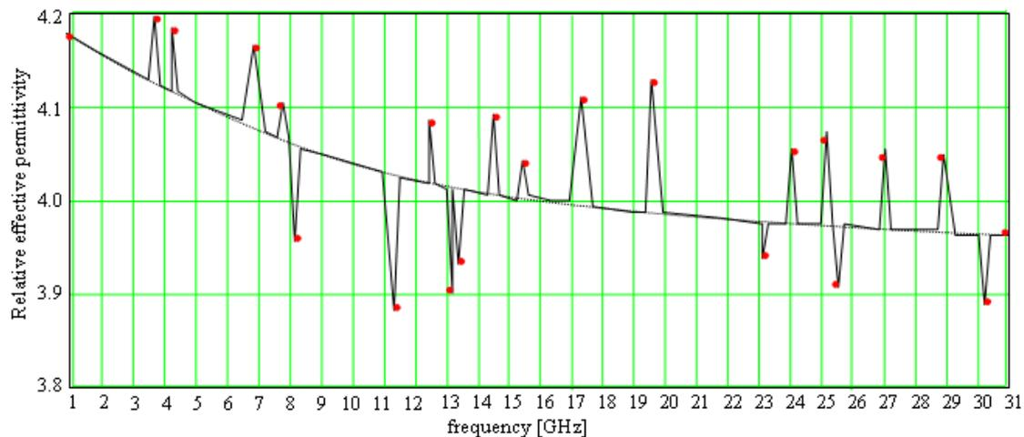
Fig. 9. The effective permittivity for the FR4 board material, calculated with our new formula for the effective permittivity of the stratified resins. All resonances obtained by simulation are illustrated on graph.
