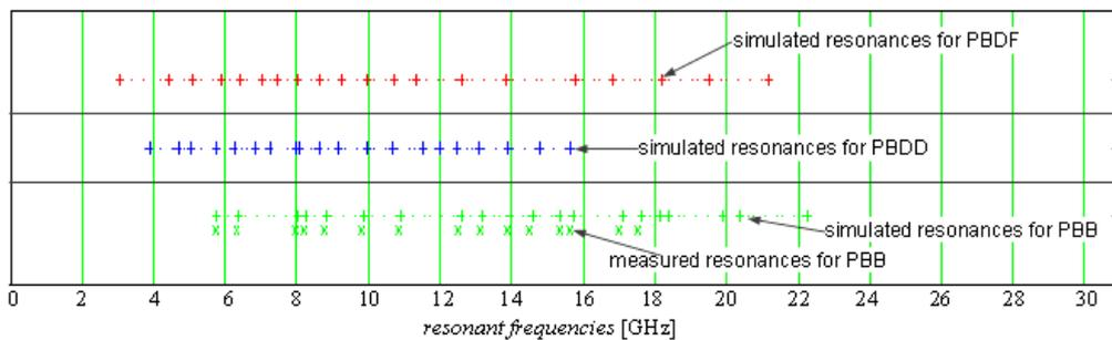
Fig. 7. Resonant frequencies for PBB, PBDD and PBDF, obtained by simulations and measurements.
