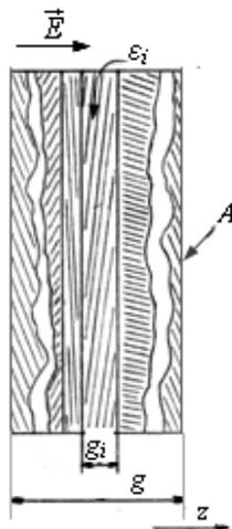
Fig. 4. Mixed dielectric material, consisting of parallel wavy layers of homogeneous dielectrics (after B. P. Scaife [8]).
