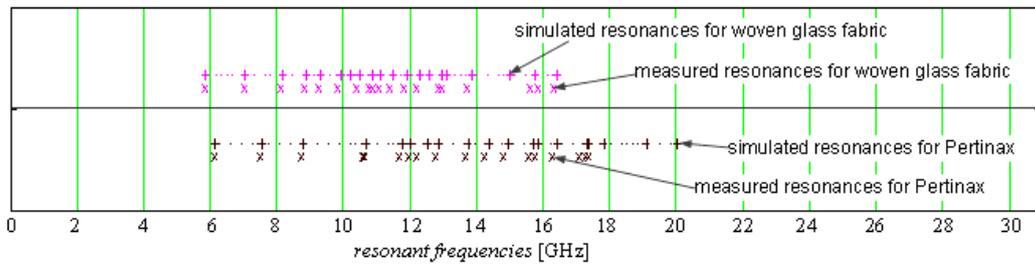
Fig. 6. Resonant frequencies for Pertinax and woven glass fabric, obtained by simulations and measurements.
