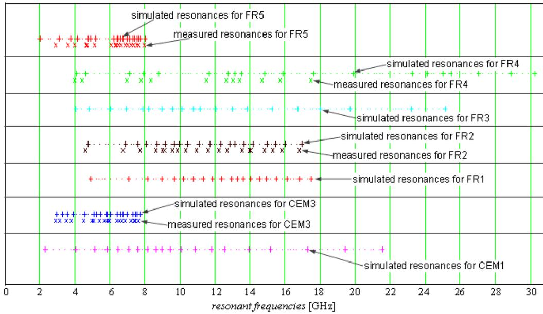
Fig. 8. Resonant frequencies for the halogen-free board materials CEM-1, CEM-3, FR1, FR2, FR3, FR4 and FR5, obtained by simulations and measurements.
