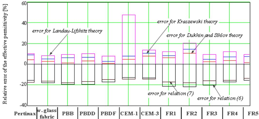
Fig. 5. The relative error of the relative effective permittivity values for the considered theories - graphical representation. One observes that the Dukhin and Sihlov theory gives the most precise results for the board materials.
