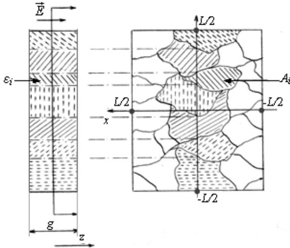
Fig. 3. Mixed dielectric material, consisting of parallel cylinders with irregular cross-sections (after B. P. Scaife [8]).
