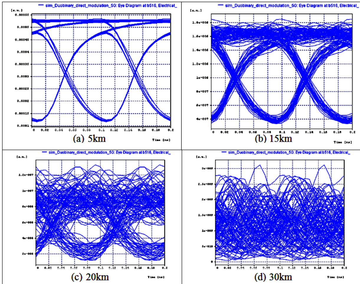
Fig. 8. Eye diagram with 5Gbps bit rate at (a) 5km; (b) 15km; (c) 20km; (d) 30km.
