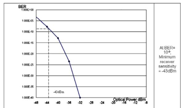
Fig. 5. BER versus receiver power sensitivity (dBm) for 1Gbps.
