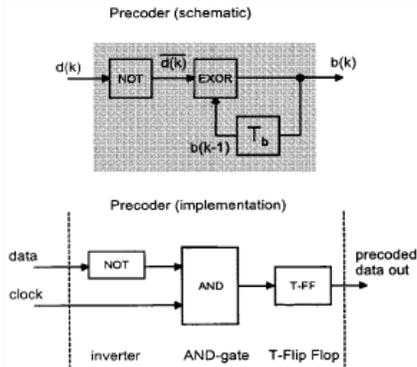
Fig. 1. Simple realization of duobinary precoder.
