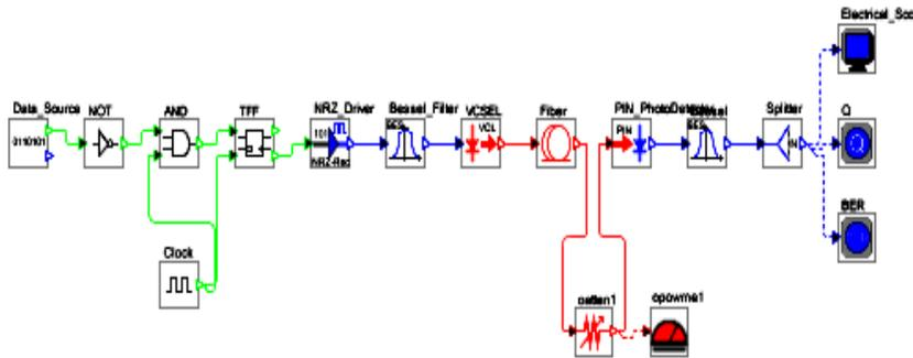
Fig. 2. Schematic setup for single-arm duobinary direct modulation format.
