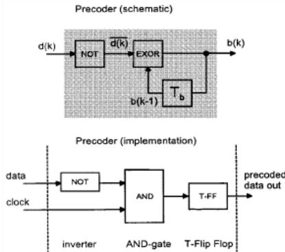
Fig. 1. Simple realization of duobinary precoder.
