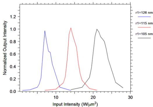
Fig. 3. The output diagram of the nonlinear PhCRR for different values of r1 (color online)
