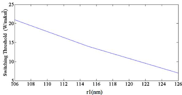
Fig. 2. The variation of the switching threshold of the nonlinear PhCRR versus r1
