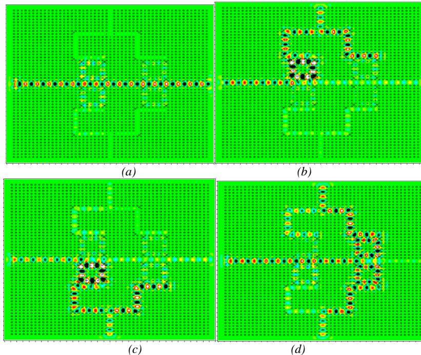
Fig. 5. The optical behavior of the proposed ASK demodulator when the input intensity is (a)  $1 \text{ W}/\mu\text{m}^2$ , (b)  $7 \text{ W}/\mu\text{m}^2$ , (c)  $14 \text{ W}/\mu\text{m}^2$  and (d)  $21 \text{ W}/\mu\text{m}^2$  (color online)
