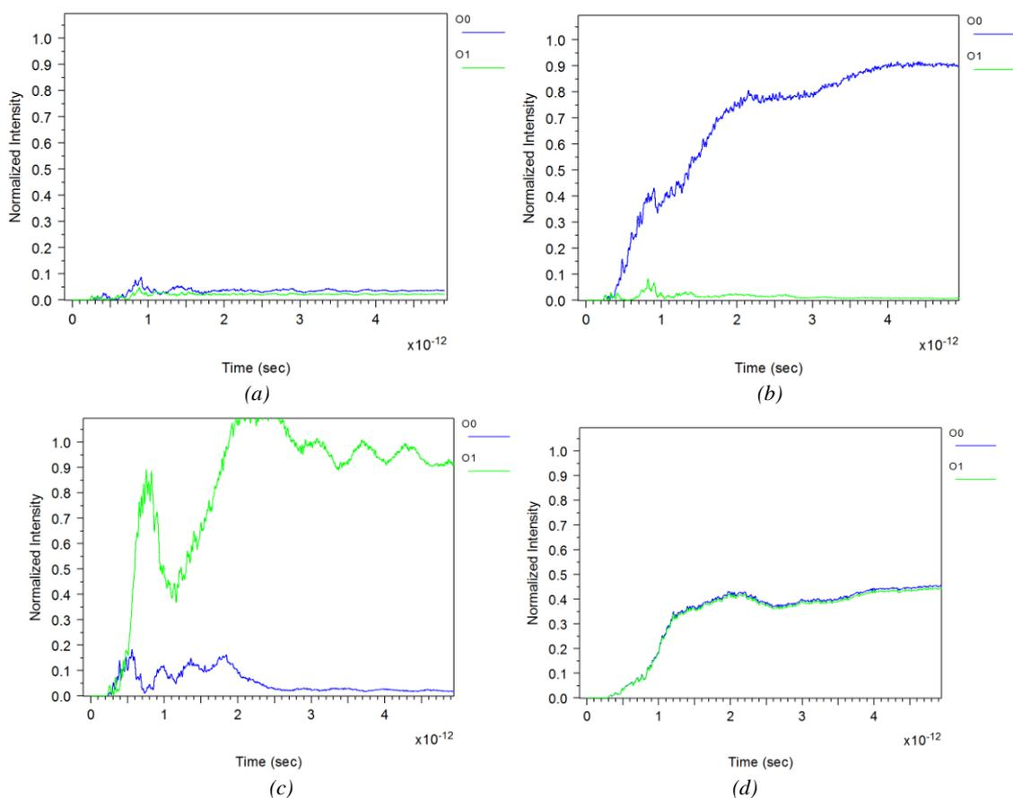
Fig. 6. The output diagram of the proposed ASK demodulator when the input intensity is (a)  $1 \text{ W}/\mu\text{m}^2$ , (b)  $7 \text{ W}/\mu\text{m}^2$ , (c)  $14 \text{ W}/\mu\text{m}^2$  and (d)  $21 \text{ W}/\mu\text{m}^2$  (color online)
