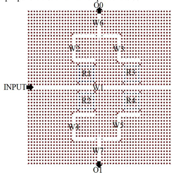
Fig. 4. The proposed optical ASK demodulator (color online)
