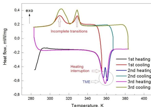
Fig.2 Heat flow variation during heating arrest before the completion of martensite reversion, causing the occurrence of temperature memory effect in subsequent heating cycle
