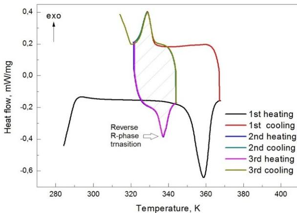
Fig.3 Heat flow variation revealing perfectly reversible R-phase transition (hatched area)
