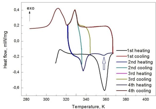
Fig.4 Heat flow variations emphasizing the absence of TME during R-phase transition
