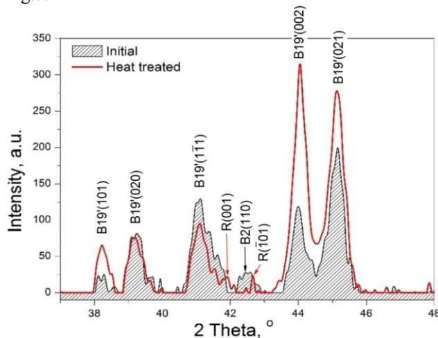
Fig.7 Magnified XRD patterns of the wire specimens in initial and heat treated conditions, emphasizing the changes induced by heat treatment.
