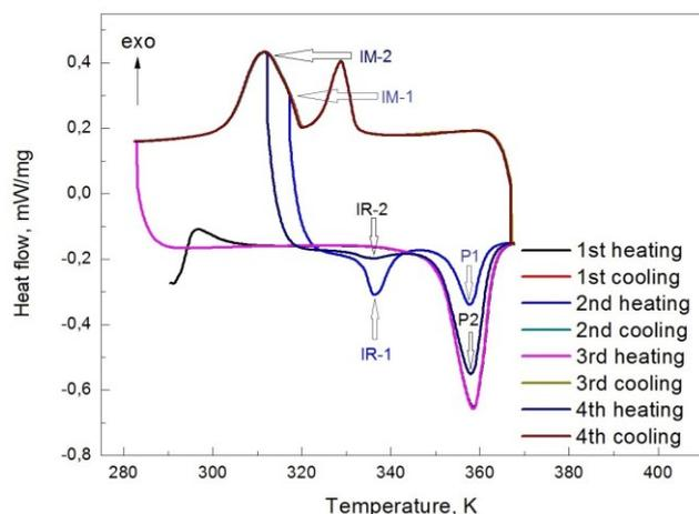
Fig.5 Heat flow variations emphasizing the competition between martensitic transformation and R-phase transition
