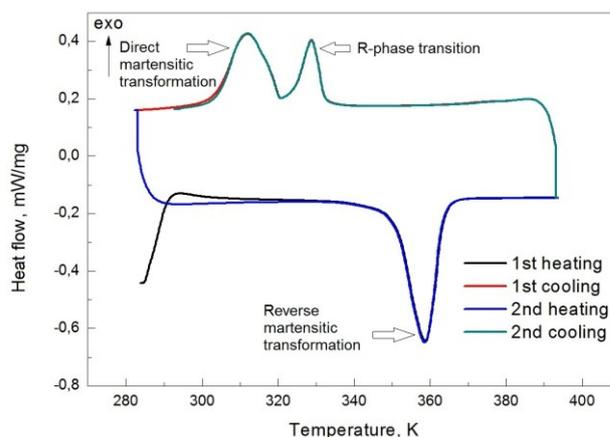
Fig.1 Heat flow variation during two stabilized heating-cooling cycles of the wire specimen in initial condition, revealing a reversible martensitic transformation and R-phase transition
