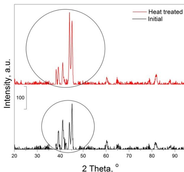
Fig.6 XRD patterns of wire specimens in initial and heat treated (370 K/ 300s/ furnace/ 333K/ water) conditions
