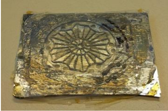
Fig. 5. Latex film glued on the microspeaker backside
