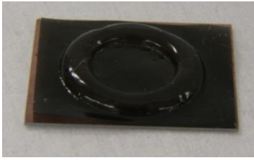
Fig. 12. Dry film applied on silicon MEMS microspeaker
