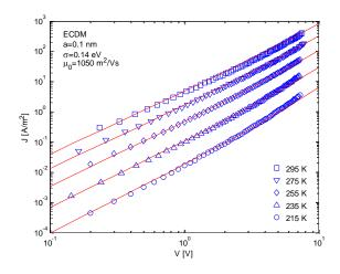
Fig. 4. Temperature dependent current density versus voltage characteristics of N2200 hole-only device with a layer thickness of 140 nm. Symbols are the experimental data from Ref. [27]. Lines are the numerically calculated results based on the ECDM.
