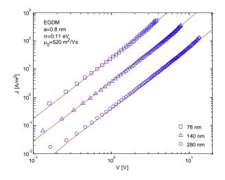
Fig. 1. Thickness dependent current density versus voltage characteristics of N2200 hole-only devices at 295K. Symbols are the experimental data from Ref. [27]. Lines are the numerically calculated results based on the EGDM.
