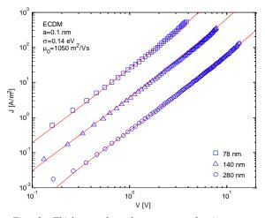
Fig. 3. Thickness dependent current density versus voltage characteristics of N2200 hole-only devices at 295K. Symbols are the experimental data from Ref. [27]. Lines are the numerically calculated results based on the ECDM.
