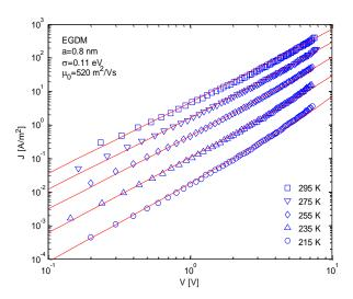
Fig. 2. Temperature dependent current density versus voltage characteristics of N2200 hole-only device with a layer thickness of 140 nm. Symbols are the experimental data from Ref. [27]. Lines are the numerically calculated results based on the EGDM.
