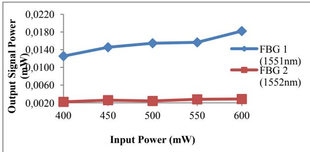
Fig. 9(a) Effect of FBG 1 and FBG 2 position for input power of system based on two wavelengths
