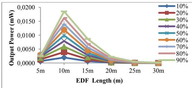
Fig. 6 Effect of EDF length for system based on two wavelengths
