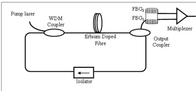
Fig. 1 Schematic design of EDFL system based on two wavelengths
