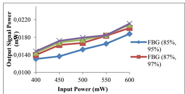
Fig. 8 Effect of different reflectivity combinations for input power of system based on two wavelengths
