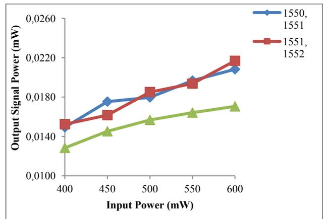
Fig. 7 Effect of different wavelength combinations for input power of system based on two wavelengths
