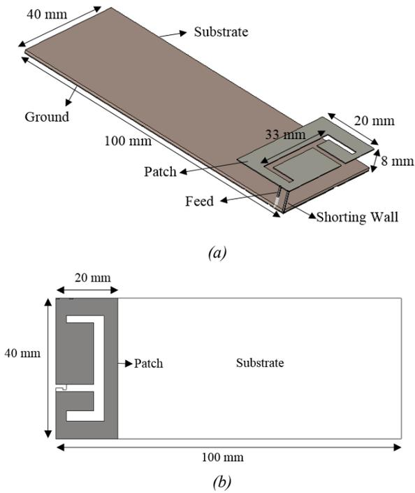
Fig. 1. Geometry of E-shaped PIFA with substrate: (a) 3D view (b) front view.
