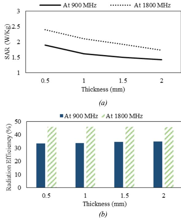
Fig. 8. PIFA with different thickness of RT Duroid substrate (a) SAR values (b) radiation efficiencies.
