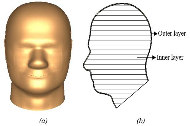
Fig. 2. SAM phantom (a) 3D view of SAM phantom, (b) Cross-section view.
