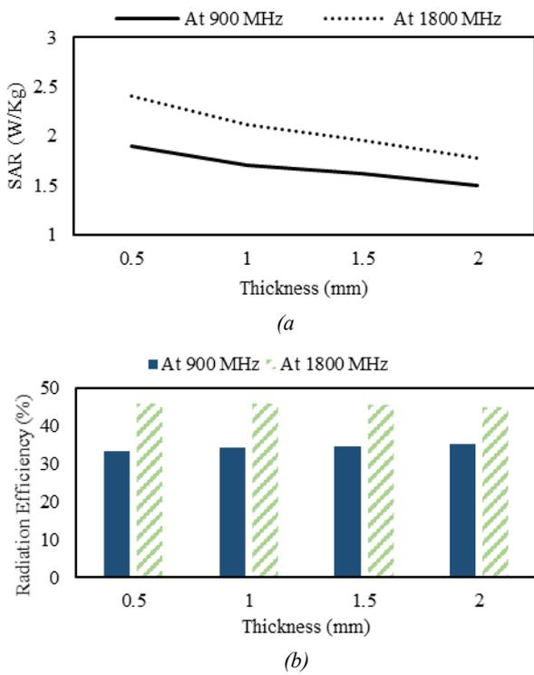
Fig. 5. PIFA with different thickness of FR-4 substrate (a) SAR values (b) radiation efficiencies.
