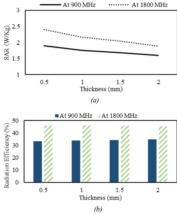
Fig. 7. PIFA with different thickness of Taconic TLC substrate (a) SAR values (b) radiation efficiencies.
