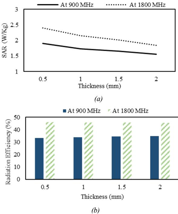
Fig. 6. PIFA with different thickness of Rogers RO4003 substrate (a) SAR values (b) radiation efficiencies.
