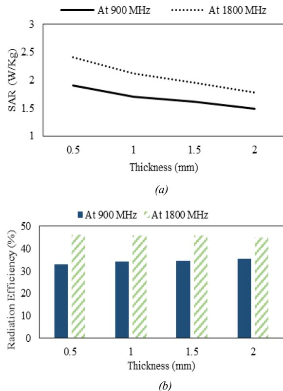
Fig. 4. PIFA with different thickness of Bakelite substrate (a) SAR values (b) radiation
