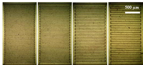
Fig. 2. Laser processed interdigital capacitors on copper film for different digit width: 20, 30, 40 and 50 \mu\text{m} .
