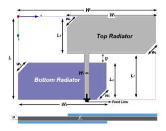
Fig. 1. Design geometry of the antenna top and crosssectional view (color online)
