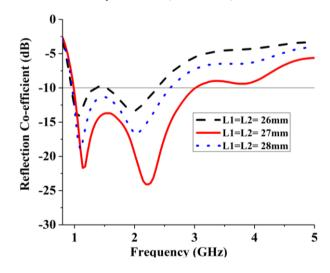
Fig. 5. Evaluation of the S11 for different length of resonators (color online)
