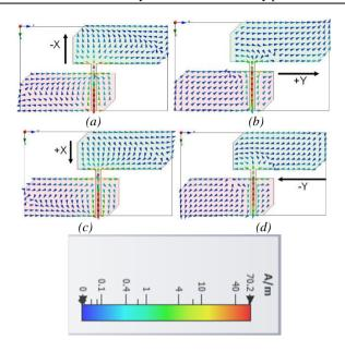
Fig. 2. Surface current distribution at (a) 0° (b) 90°(c) 180° and (d) 270° (color online)
