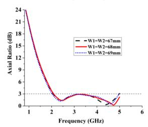
Fig. 4. Evaluation of axial ratio (AR) for different width of resonators (color online)
