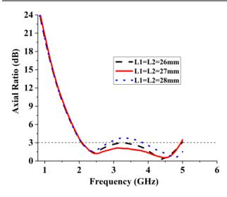
Fig. 6. Evaluation of axial ratio (AR) for different length of resonators (color online)
