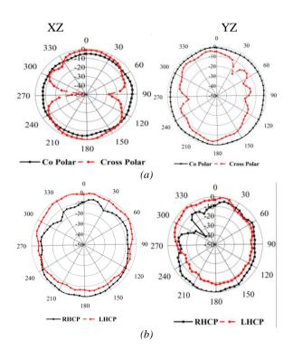
Fig. 12. Radiation pattern at (a) 1.2 GHz (Linear Polarization); (b) 2.1 GHz (Circular polarization) (color online)
