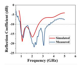
Fig. 9. Simulated and Measured Reflection Co-efficient of the proposed prototype (color online)
