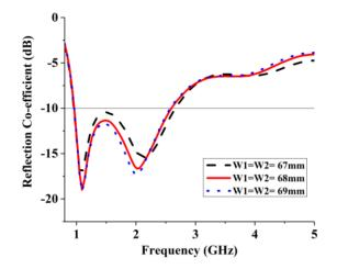
Fig. 3. Evaluation of the S<sub>11</sub> for different width of resonators (color online)
