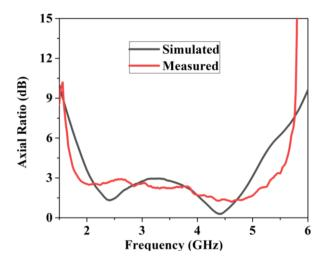
Fig. 10. Simulated and measured axial ratio bandwidth (color online)
