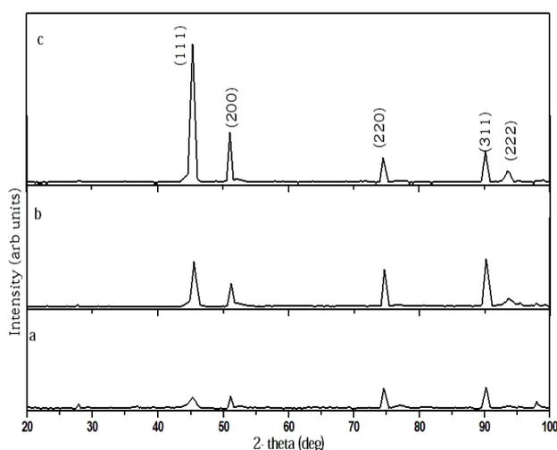
Fig. 2. XRD patterns of Ni-Mn thin film at various temperatures (a) 30°C, (b) 50°C and (c) 70°C.
