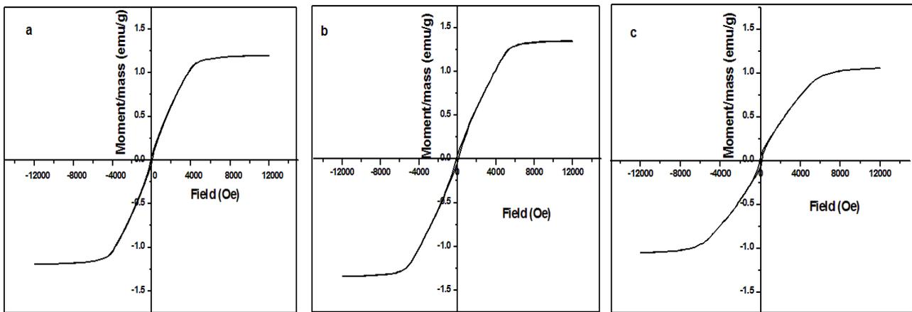
Fig. 6. Magnetic Hysteresis loop of the electrodeposited Ni-Mn film at various temperature (a) 30°C, (b) 50°C and (c) 70°C.
