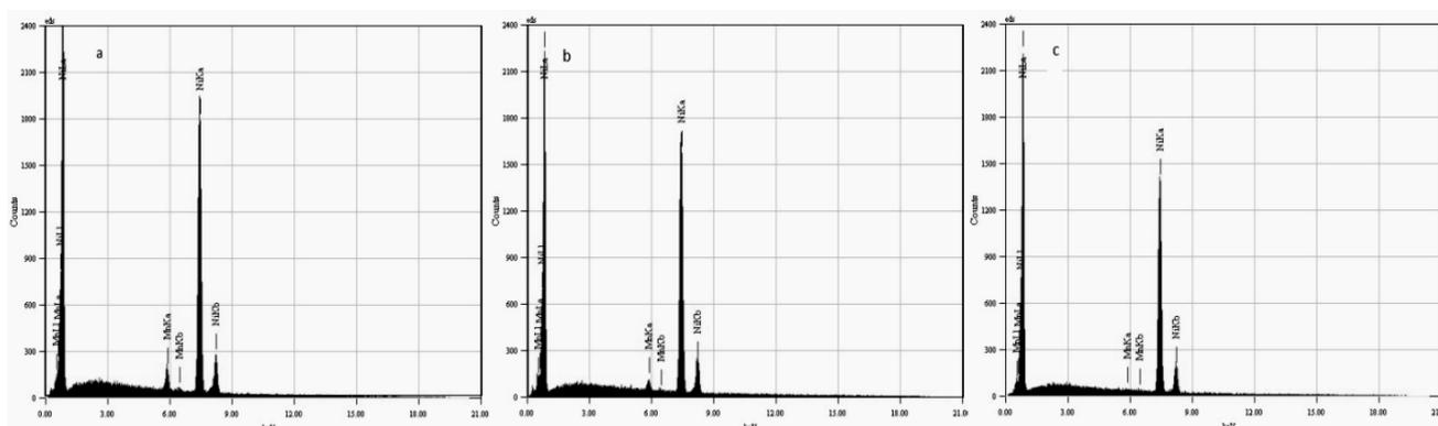
Fig. 1. EDAX spectrum of Ni-Mn thin film at various temperature (a) 30°C, (b) 50°C and (c) 70°C.
