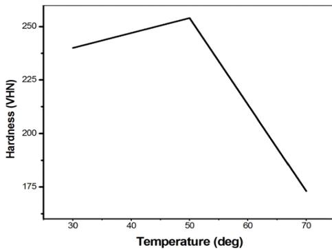
Fig. 5. Effect of temperature on hardness of Ni-Mn thin film at various temperature.
