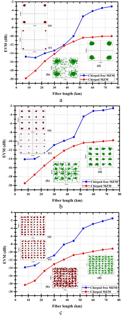
Fig. 2.  $EVM$  performance analysis for different fiber lengths for (i) 4QAM, (ii) 16QAM, (iii) 64QAM. Inset (a,c for chirp free and chirped OFDM respectively) Constellation at distance 7.5kms (b,d for chirp free and chirped OFDM respectively) Constellation at distance 75km
