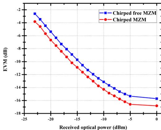
Fig. 4. EVM performance to analyze receiver sensitivity
