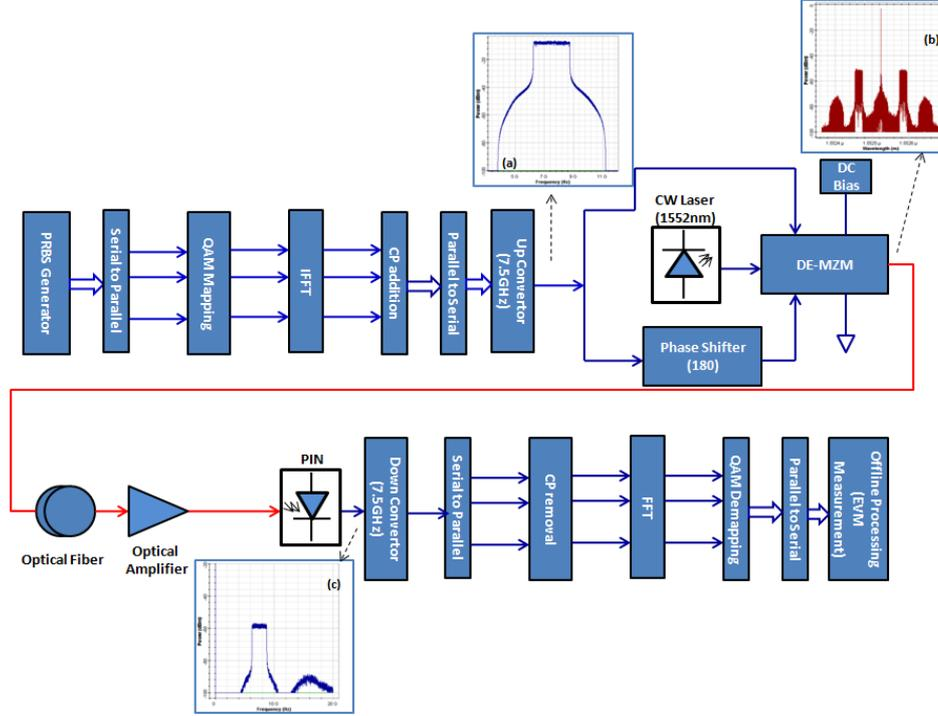
Fig.1. Optical OFDM MMW Generation with Direct Detection. (a) OFDM spectrum after up conversion. (b) Optical OFDM DSBFC spectrum. (c) Photodetected RF spectrum
