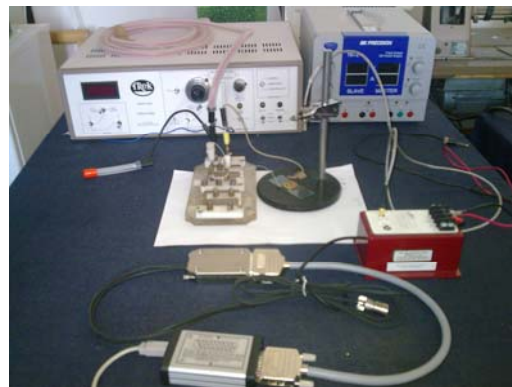
Fig. 2. Experimental setup for field-induced thickness strain measurements.
