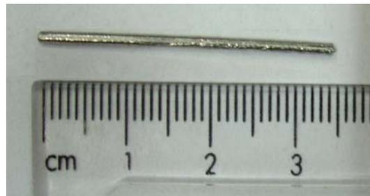
*Fig. 1. Amorphous rod obtained by copper mould casting.*
