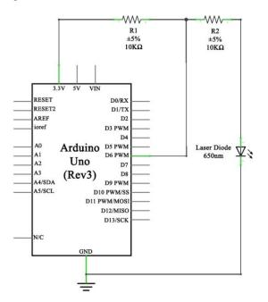
Fig. 16. Transmitter circuit diagram
