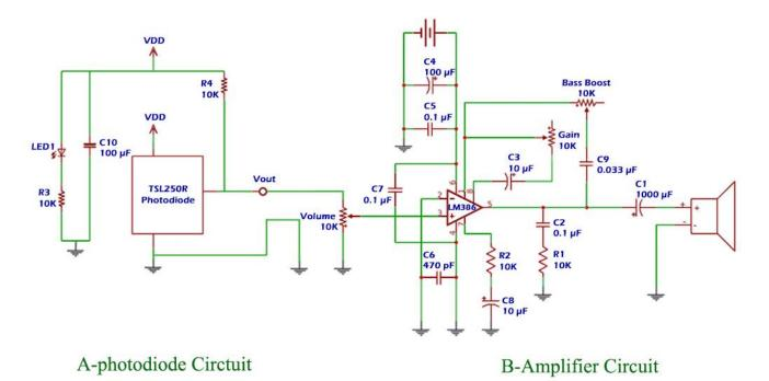
Fig. 4. Received circuit design (photodiode circuit plus an audio amplifier circuit)
