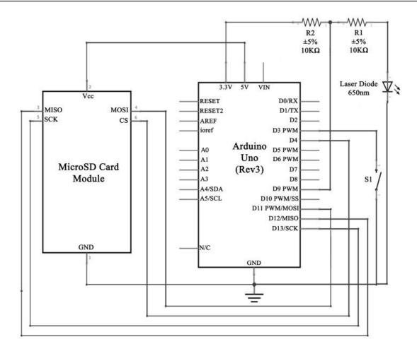
Fig. 2. Transmitter circuit design
