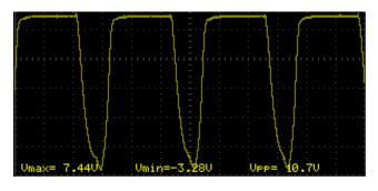
Fig. 9. Received audio signal after being amplified
