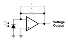
Fig. 5. TSL250R functional block diagram [8]
