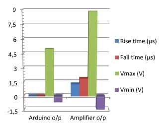
Fig. 12. A comparison between using the Arduino and the LM386 amplifier circuit after receiving the signal
