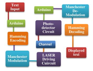
Fig. 18. Model operational steps diagram
