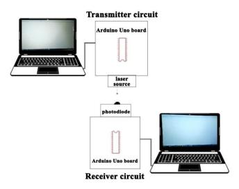
Fig.15. Text transmission implemented model diagram
