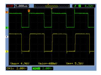
Fig. 14. Transmitted and received signals using Arduino board
