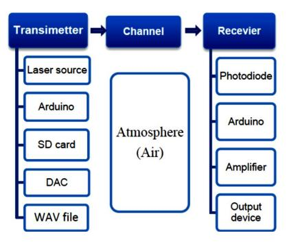
Fig. 1 Audio system configuration
