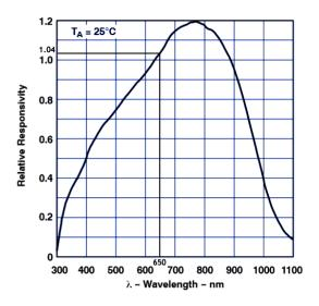
Fig. 6. TSL250R photodiode spectral responsivity [8]
