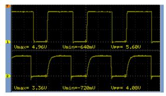
Fig. 11. Comparison between the received signals using the Arduino (1) vs. not using the Arduino (2)
