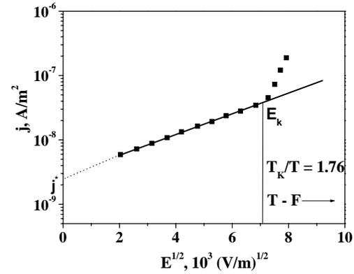
Fig. 4.  $V$ - $A$  characteristic in Schottky coordinates.
