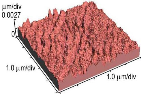
Fig. 3. AFM 3D image of an  $(As_2S_3)_{90}(AgI)_{10}$  thin film.
