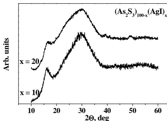
Fig. 1. X-ray diffraction patterns for some glass compositions of the  $(As_2S_3)_{100-x}(AgI)_x$  system.
