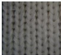
Jersey fabric – real aspect (front), knitting sequence and symbolic representation
