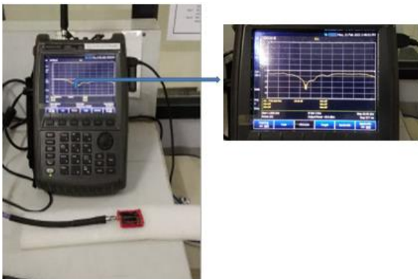
Fig. 7. Fabricated Antenna mounted on VNA (Vector Network Analyzer) (color online)
