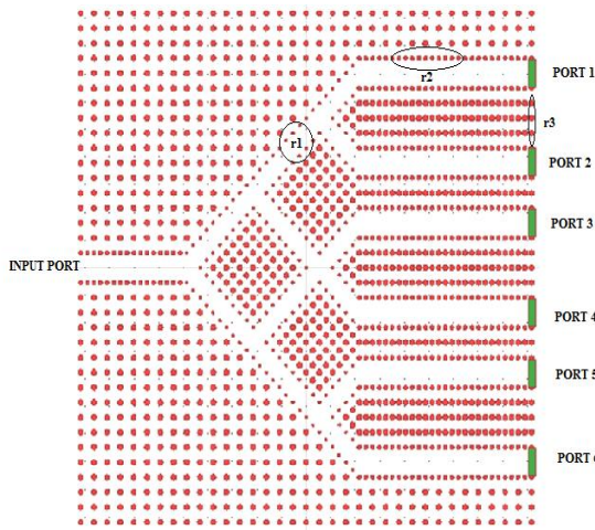
Fig. 11. Structural design of 1x6 power splitter
