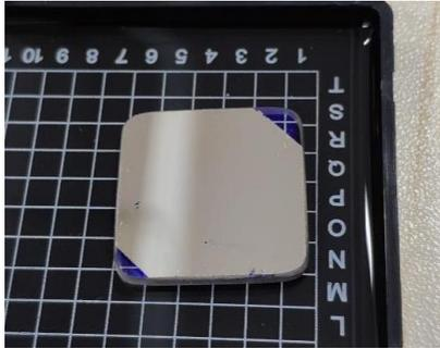
Fig. 7. Sample of an Al film obtained by magnetron sputtering (color online)
