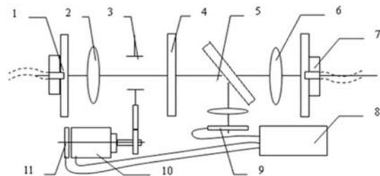
1, 7- Optical fiber coupler; 2-Collimating lens; 3- Iris diaphragm;
