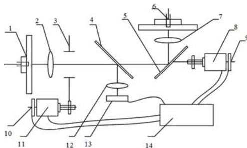
1、 6-Optical fiber coupler; 2-Collimating lens; 3-Iris diaphragm;
