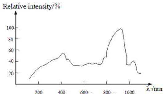
Fig. 2. The spectrogram of the system's light source.
