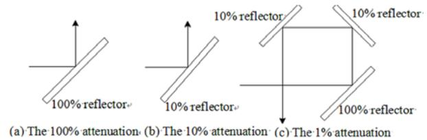
Fig. 5. The 3 kinds of attenuations of the reflector attenuation array.
