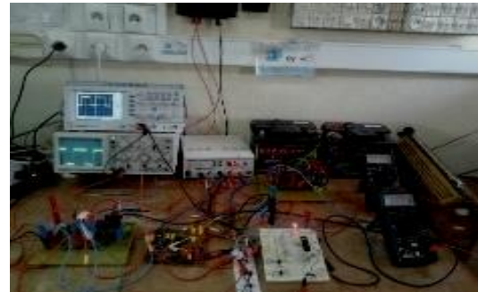
Fig. 12. PV panels type SP75, test bench used in the laboratory, DC/DC Boost converter and digital MPPT control.
