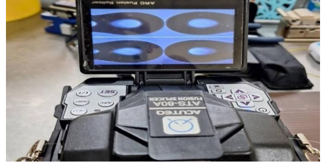
Fig. 1. Formation of microresonators from single-mode fibers using a fusion splicer (colour online)
