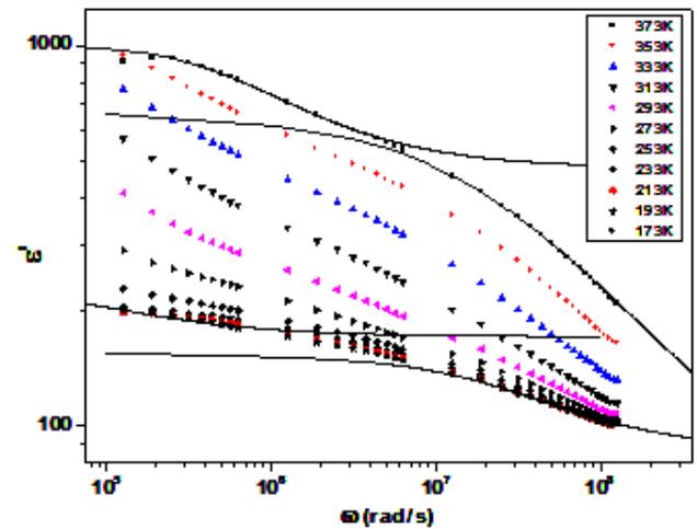
Fig. 3. Variation of the dielectric constant with frequency at different temperatures
