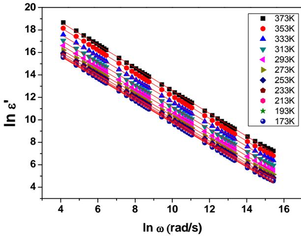
Fig. 5. Variation of the dielectric loss with frequency at different temperatures
