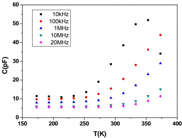
Fig. 2. Temperature dependence of capacitance at different frequencies
