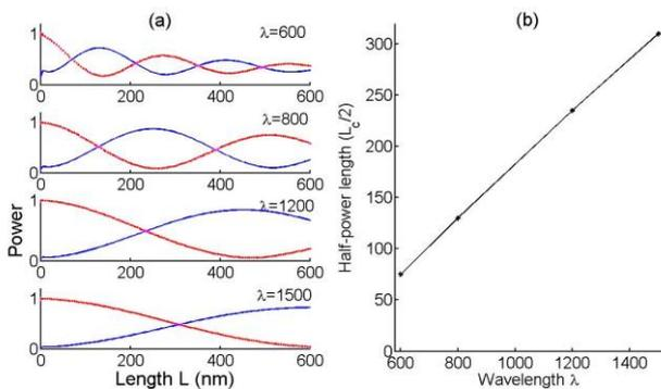
Fig. 2. (a) Power exchange between the waveguides of the plasmonic coupler along the waveguide length  $L$  at different wavelength for silver-air interface. (b) Variation of half-power Length  $L_c/2$  with wavelength (color online)
