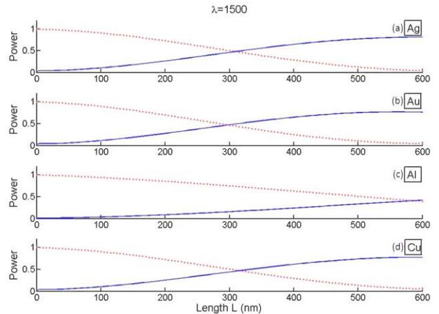
Fig. 3. Power exchange between the waveguides of the plasmonic coupler along the waveguide length for different metal-air interface at wavelength  $\lambda = 1500$  nm (color online)
