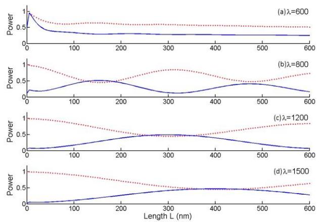
Fig. 13. Coupling dynamics in Ag-air-Ag-glass-Ag plasmonic coupler. Waveguide-1 is now filled with air, while the other is with glass  $n=1.5$ . Rest of the parameters are as in Fig. 12 (color online)
