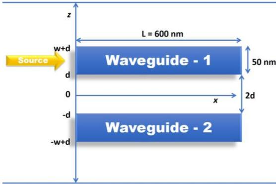
Fig. 1. Schematic diagram of MIMIM plasmonic coupler (color online)
