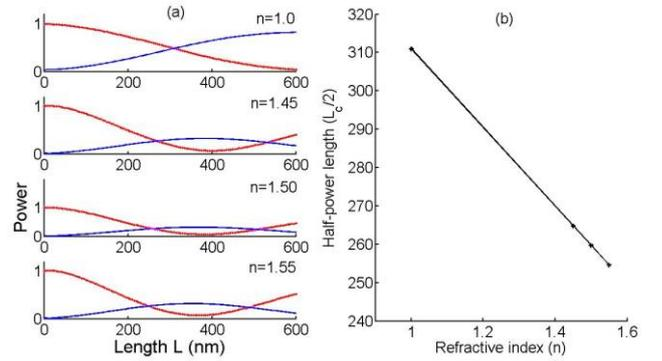
Fig. 8. (a) Variation of power in the Ag-glass-Ag-glass-Ag coupler along the waveguide length 'L' for glasses of different refractive indices 'n' at  $\lambda = 1500$  nm. (b) Variation of half-power length (or  $L_c/2$ ) with refractive index (color online)
