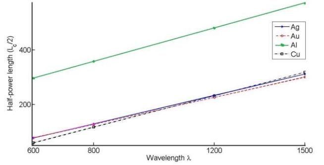
Fig. 7. Variation of half-power length  $L_c/2$  with wavelength for Ag, Au, Al and Cu (color online)
