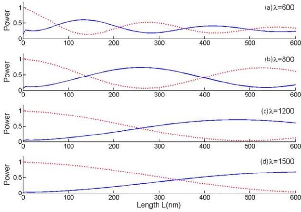
Fig. 10. Power coupling dynamics with waveguide-1 of thickness 50 nm and waveguide-2 of thickness 60 nm, i.e., the thickness of the power launching waveguide is now narrower. Rest of the parameters as in Fig. 9 (color online)
