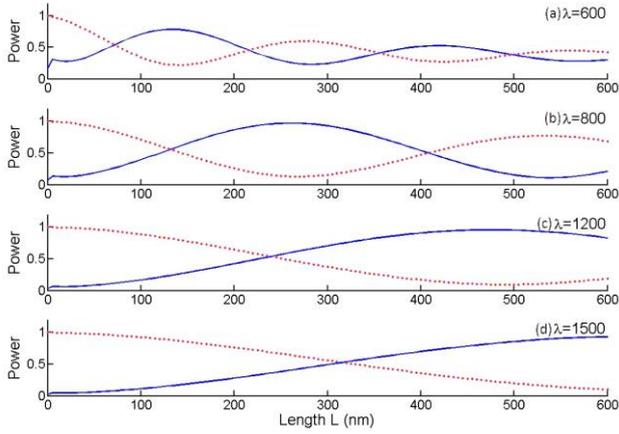
Fig. 9. Power coupling dynamics with waveguide-1 of thickness 60 nm and waveguide-2 of thickness 50 nm (color online)
