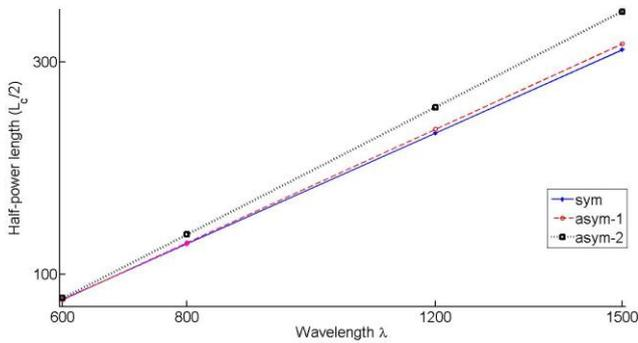
Fig. 11. Comparison of the dependence of half-power length  $L_c/2$  on wavelength for (a) symmetric (b) and (c) Asymmetric (color online)
