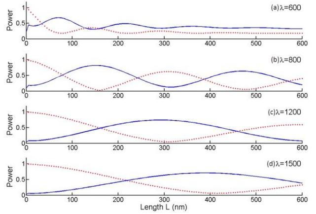
Fig. 12. Coupling dynamics in Ag-glass-Ag-air-Ag plasmonic coupler. Waveguide-1 is of glass  $n=1.5$  and waveguide-2 is air-filled  $n=1$  (color online)
