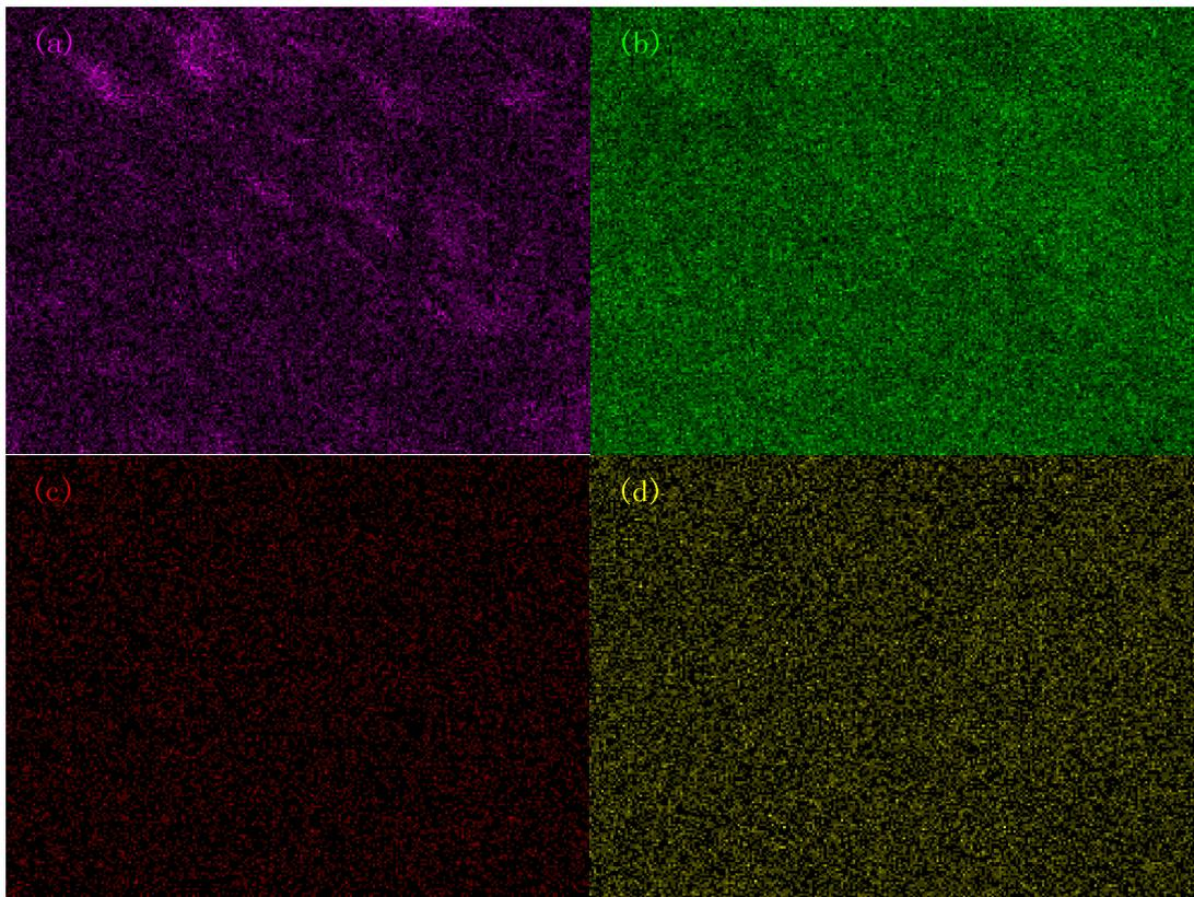
Fig. 4. Elemental mapping images of the representative sample E: (a) Zn, (b) O, (c) Ag and (d) Al (color online)
