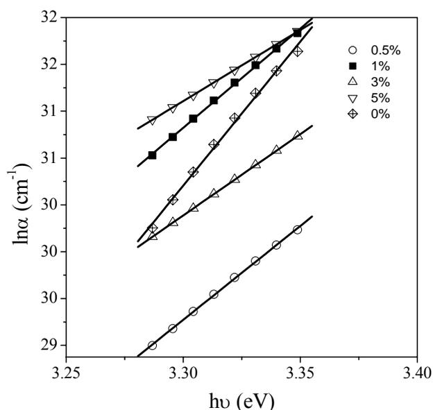
Fig. (4). Variation of  $\ln(\alpha)$  as a function of photon energy ( $h\nu$ ) for three dimensional ZnO thin films doped with different Al concentrations.
