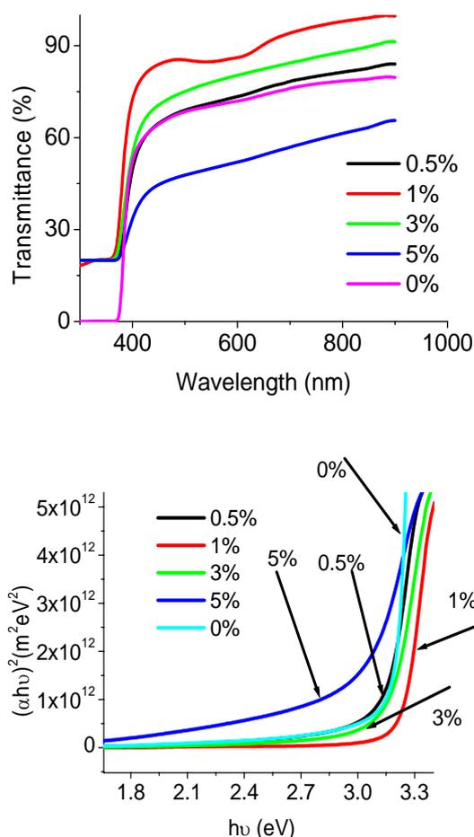
Fig. 3 (a) Optical Transmittance spectra at room temperature of undoped ZnO and AZO thin film (b)  $(\alpha h\nu)^2$  vs.  $h\nu$  curve for undoped ZnO and AZO thin film.
