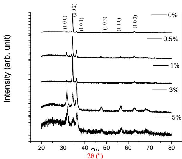
Fig. 1. XRD spectra of undoped ZnO and AZO film deposited on glass substrate at  $380^\circ\text{C}$  for various Al Doping concentrations.
