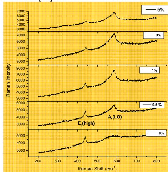
Fig.(7) Room Temperature Raman spectra of AZO film deposited on glass substrate at various Al doping concentrations.
