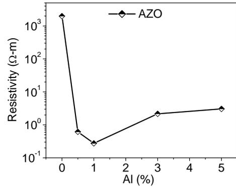
Fig.6 Electrical resistivity of undoped and AZO films deposited at 380°C as a function of Al doping concentration.
