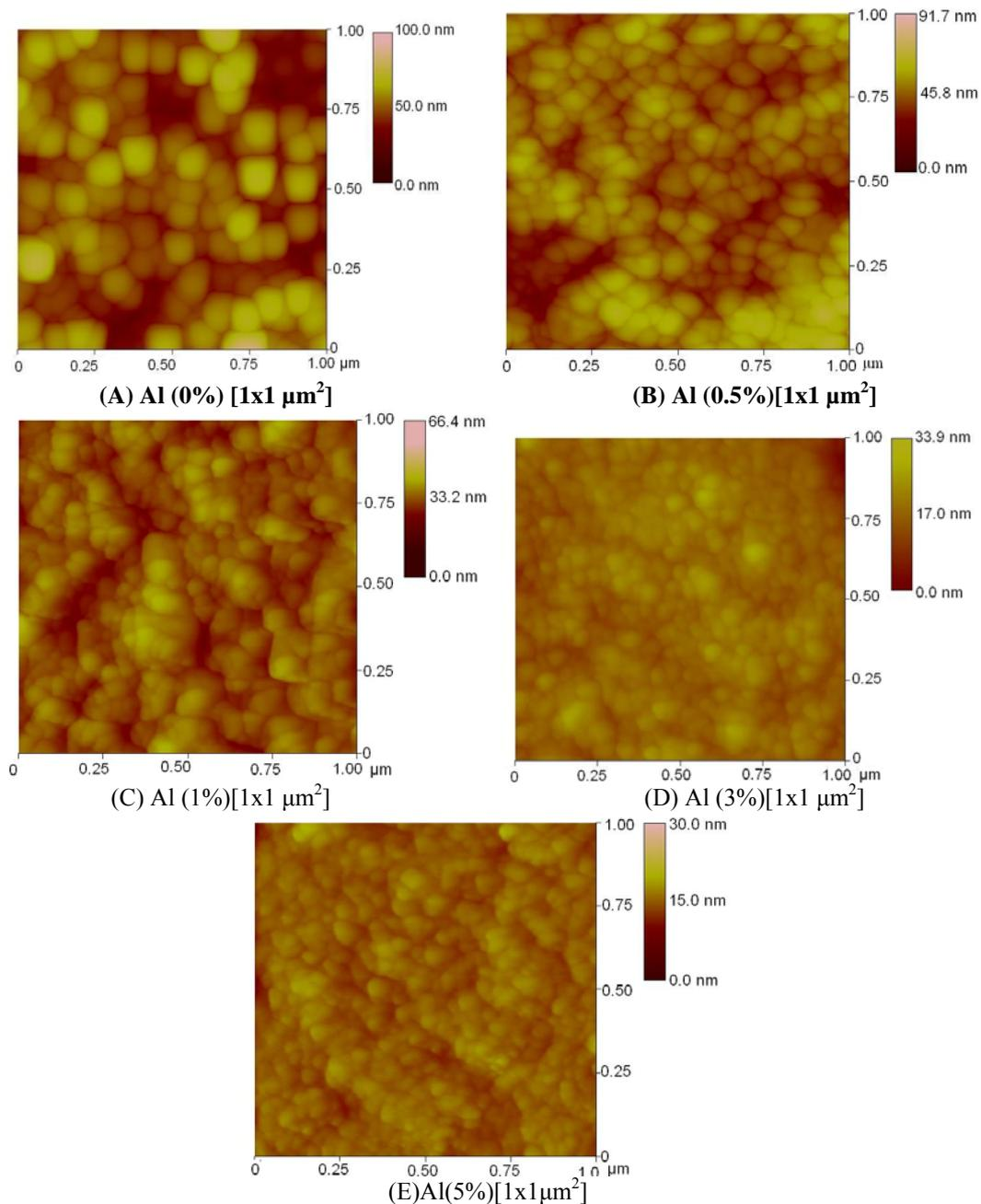
Fig. 2. Two dimensional atomic force micrograph of AZO film at various Al concentration: (a) 0% (b) 0.5% (c) 1% (d) 3% (e) 5%
