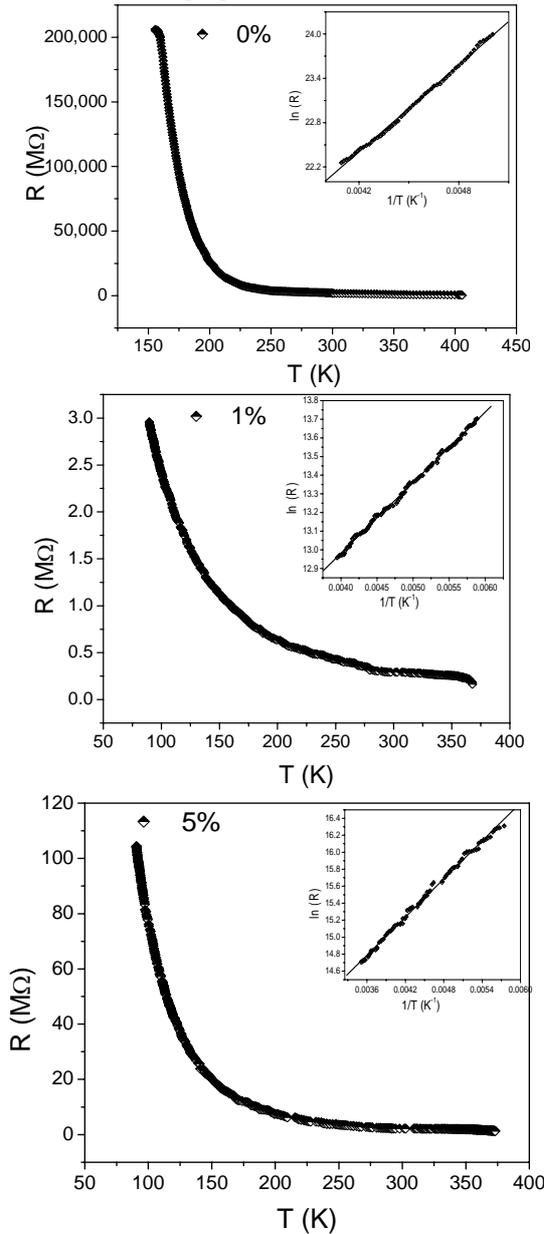
Fig. 5. Resistance vs temperature curve for Undoped and Al doped ZnO thin film at (a) 0% (b) 1% (c) 5%.
