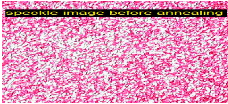
Fig. 3. Speckle image of films as deposited (color online)
