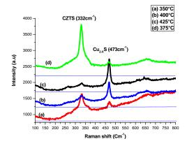
Fig. 3.Raman spectra of thin CZTS for  $T = 350^{\circ}C$ , 375°C, 400°C and 425°C.
