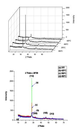
Fig.1. XRD patterns of CZTS samples prepared at different temperatures.
