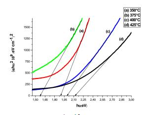
Fig.4 Variation of (atu)<sup>2</sup> with the incident photon energy from the transmission for samples prepared at different temperatures.
