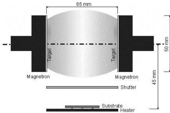
Fig. 1. Magnetron sputtering system
