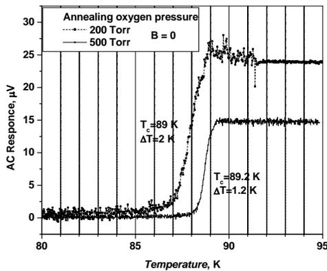
Fig. 4. Temperature dependence of the amplitude of the basic harmonic of the response signal of YBCO films exposed to the action of an AC magnetic field ( $<0.01$  mT). A decrease in the response signal amplitude starts at  $T = T_c = 89$  and 89.2 K, for the samples annealed at 200 and 500 Torr oxygen pressures respectively.
