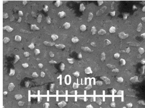
Fig. 5. Surface morphology of a YBCO film annealed at 500 mbar oxygen pressure.
