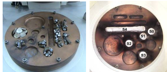
Fig. 2. Preparation of metallic charge for VAR equipment and metallic samples.
