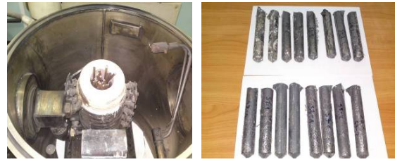
Fig. 1. Obtainment of microalloyed steels in the VIM furnace and metallic samples.
