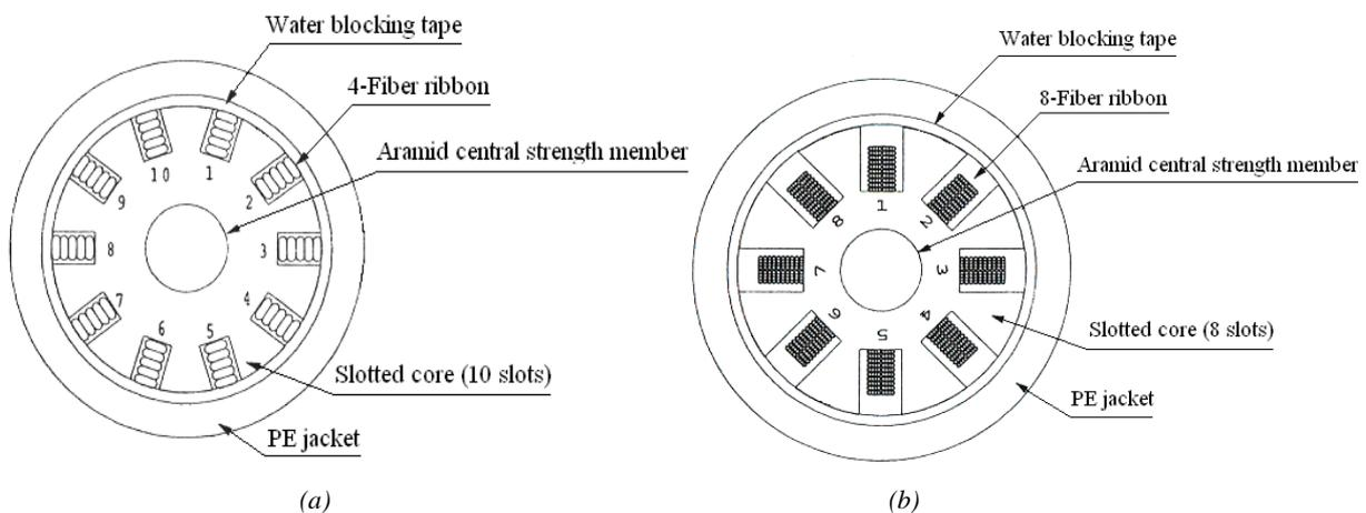
Fig. 1. a) Structure of Cable 1 (200-fiber, 10 slots, 5 layers of 4-fiber ribbons) and b) Structure of Cable 2 (640-fiber, 8 slots, 10 layers of 8-fiber ribbons)
