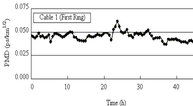
Fig. 3. Variation of PMD with ambient temperature change observed in the first ring of Cable 1
