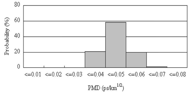
Fig. 8. Distribution of PMD values for Cable 2 in field simulation experiment
