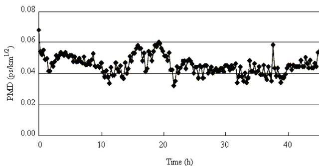
Fig. 7. Variation of PMD with ambient temperature change for Cable 2 observed in field simulation experiment
