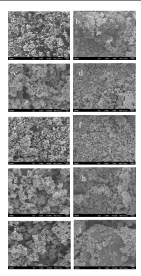
Fig. 6. SEM of ZnO/graphene and ZnO corrosion under different pH conditions (a. ZnO under pH=3; b. ZnO/ graphene under pH=3; c. ZnO under pH=5; d. ZnO/ graphene under pH=5; e. ZnO under pH=7; f. ZnO/ graphene under pH=7; g. ZnO under pH=9; h. ZnO/ graphene under pH=9; i. ZnO under pH=11; j. ZnO/ graphene under pH=11)
