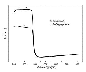
Fig. 4. UV-vis spectrum (a) ZnO; (b) ZnO/grapheme
