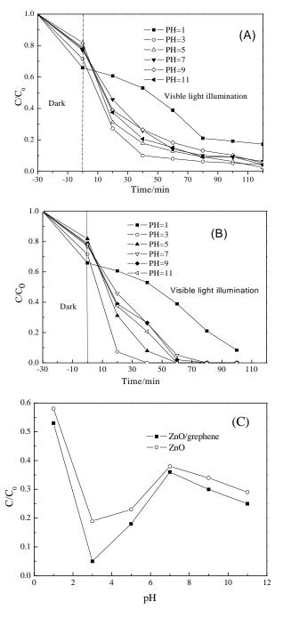
Fig. 5. Photocatalytic degradation of methyl orange under different pH conditions (A) by pure ZnO (B)by ZnO/ graphene (C) by pure ZnO and ZnO/ graphene
