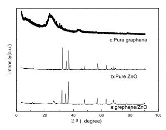
Fig. 2. X-ray diffractograms (a) ZnO/graphene, (b) ZnO, (c) Graphene
