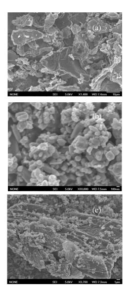
Fig. 3. SEM diagram (a) graphene (b) ZnO (c) ZnO/grapheme
