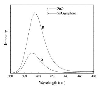
Fig. 9. Photoluminescence spectra of ZnO/graphene and ZnO
