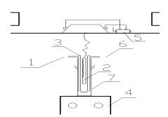
Fig. 1. The photocatalytic reactor (1 Intake; 2 300 xenon lamp; 3 Quartz liner; 4 Agitator; 5 Transformer; 6 Outfall; 7 Glass cover Fig. 1 The photocatalytic reactor)
