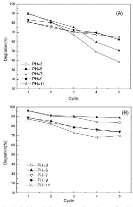
Fig. 7. Stability of photocatalytic degradation of methyl orange (A) ZnO; (B) ZnO/ grapheme
