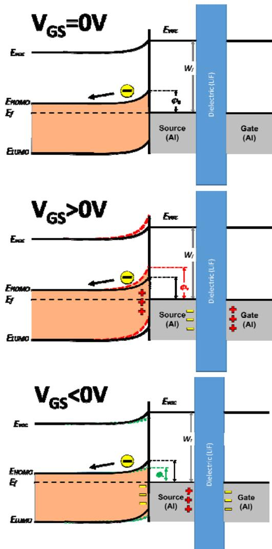
Fig. 5. Schematic diagram of energy band alignment at MEH-PPV/source/dielectric/gate of VOLETs at the different gate voltage
