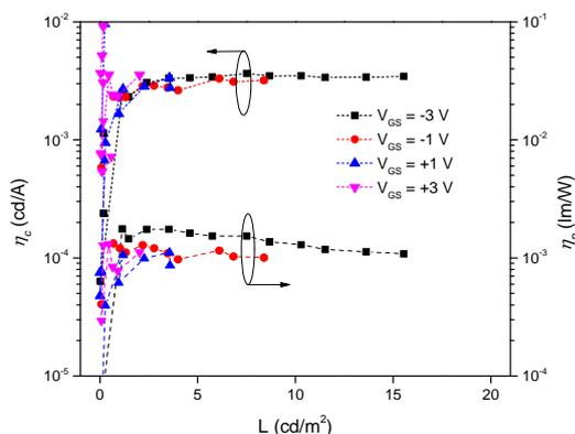
Fig. 7. Efficiencies of VOLETs at different gate voltage.
