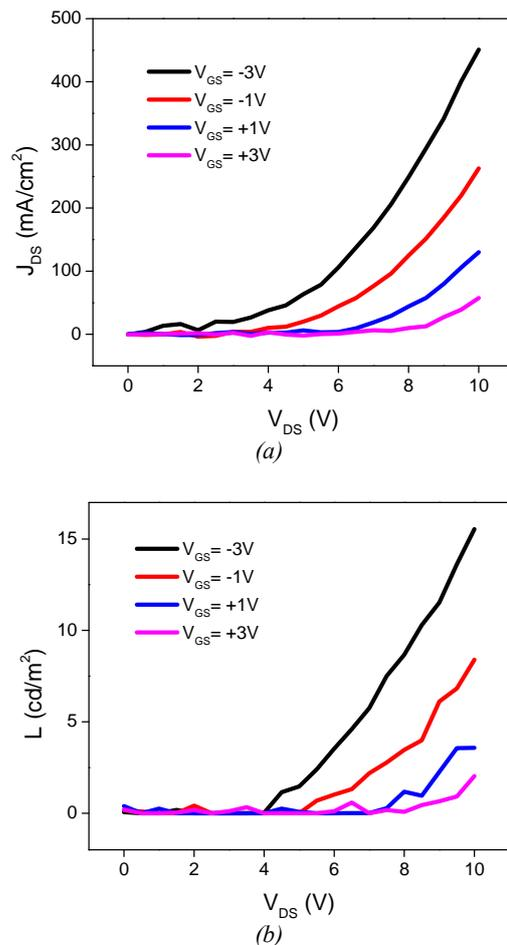
Fig. 2. Output (a) current and (b) luminance of VOLETs
