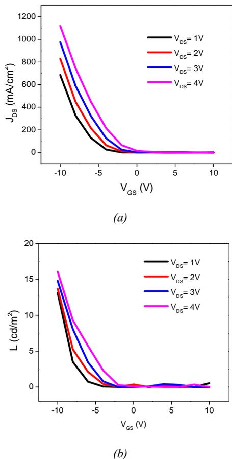
Fig. 6. Transfer characteristics of the VOLETs.
