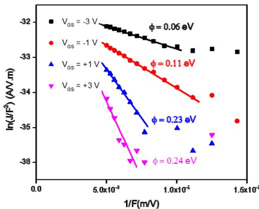
Fig. 4. FN plot of VOLETs at the different gate voltage.
