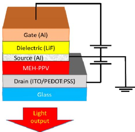
Fig. 1. Device architecture of VOLETs fabricated in this work
