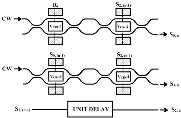
Fig. 3. Electro-optical design for LN-MZI based CRC decoder circuit
