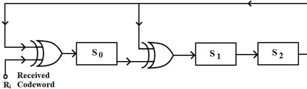
Fig. 2. (7, 4) CRC decoder logic diagram for generator polynomial  $G(x) = 1011$
