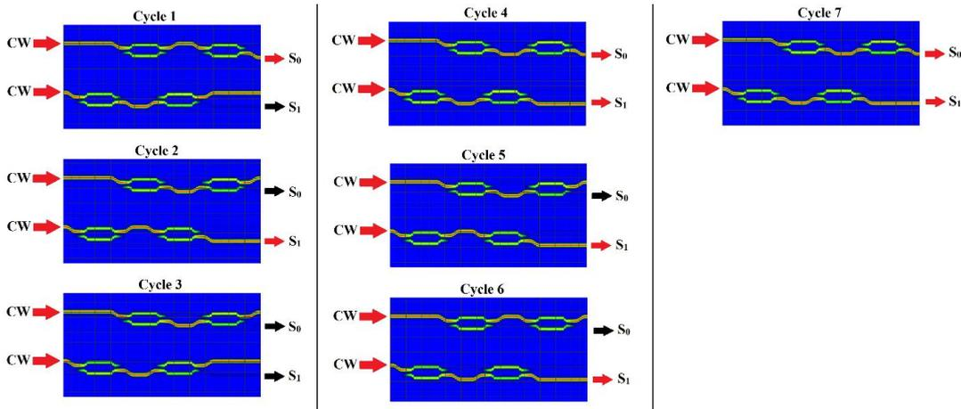
Fig. 4. Opti-BPM simulation of (7, 4) CRC decoder for received code word = 100010,  $S_2S_1S_0 = 111$ , error at  $R_5$  (color online)
