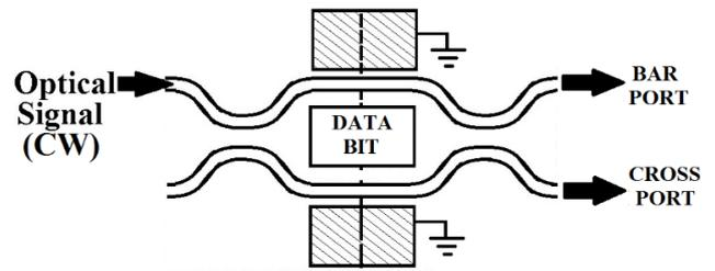
Fig. 1. Ti: LiNbO<sub>3</sub> based Mach-Zehnder interferometer
