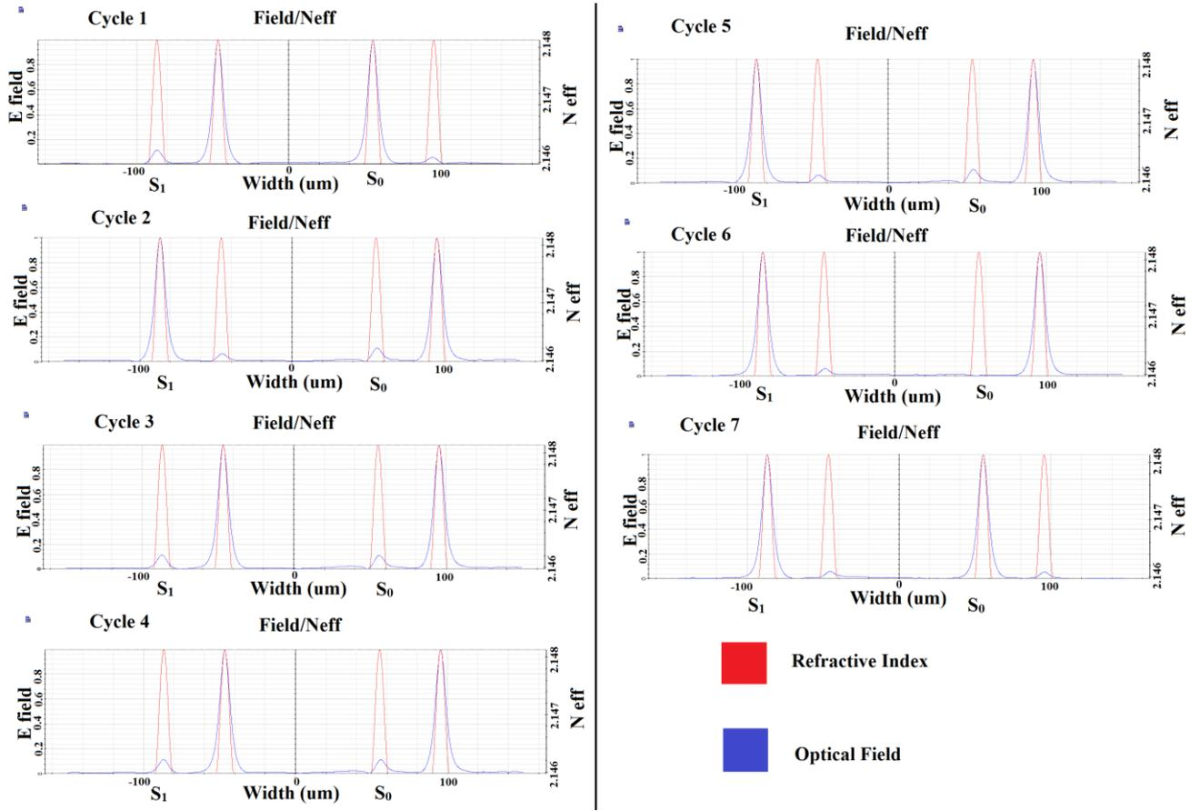
Fig. 5. Variation of optical field and refractive index at the output plane (color online)
