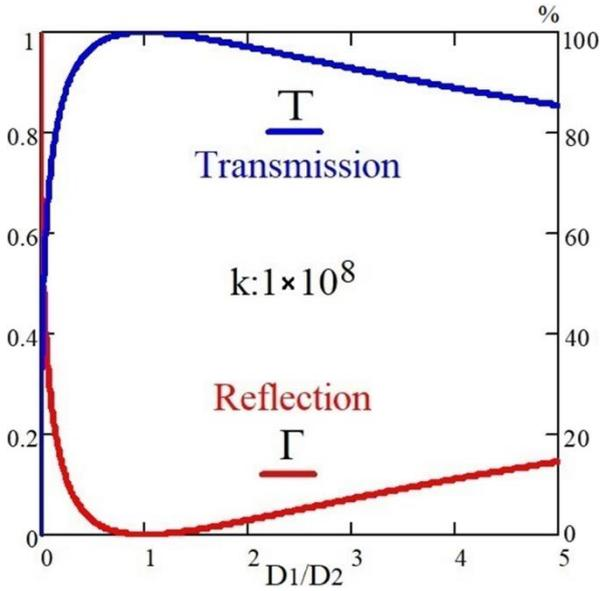
Fig. 7. The correlation between transmission and reflection based on the ratio of material parameter ratios (color online)
