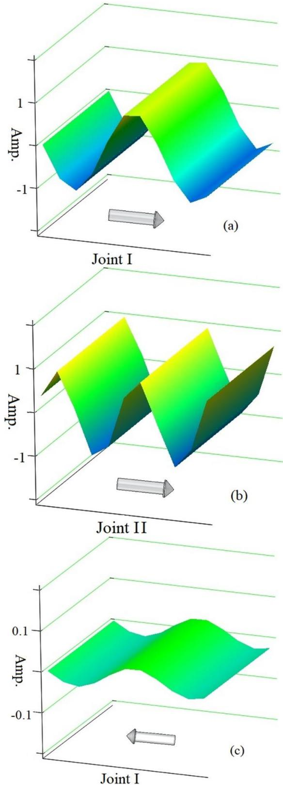
Fig. 8. Waveforms regarding EM wave propagation in the conjoined carbon nanotube, (a) the incident EM wave, (b) the transmitted EM wave, and (c) the reflected, backward EM wave (color online)
