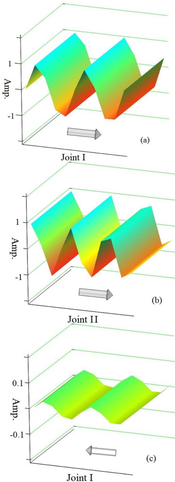
Fig. 9. Waveforms regarding EM wave propagation in the conjoined macro structure, (a) the incident EM wave, (b) the transmitted EM wave, and (c) the reflected, backward EM wave (color online)
