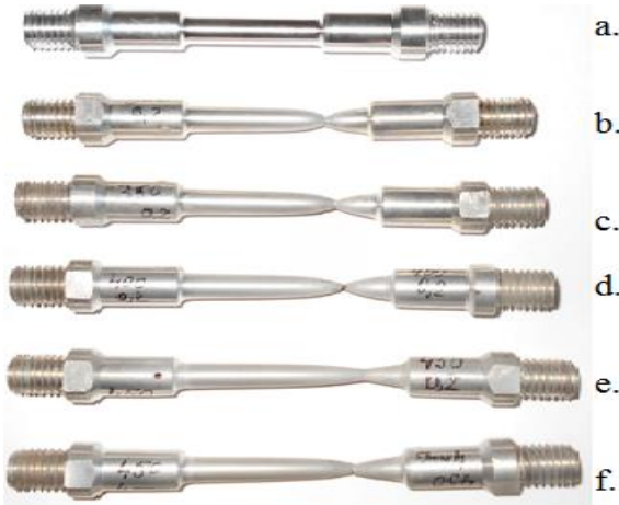
Fig. 3. Specimens tested in tension : a) initial specimen; b) T= 300 °C, ε̇=0,005 s -1 ; c) T= 350°C, ε̇=0,005 s -1 , d) T= 400 °C, ε̇=0,005 s -1 , e) T= 450 °C, ε̇=0,005 s -1 , f) T= 450°C , ε̇=0,1 s -1 .
