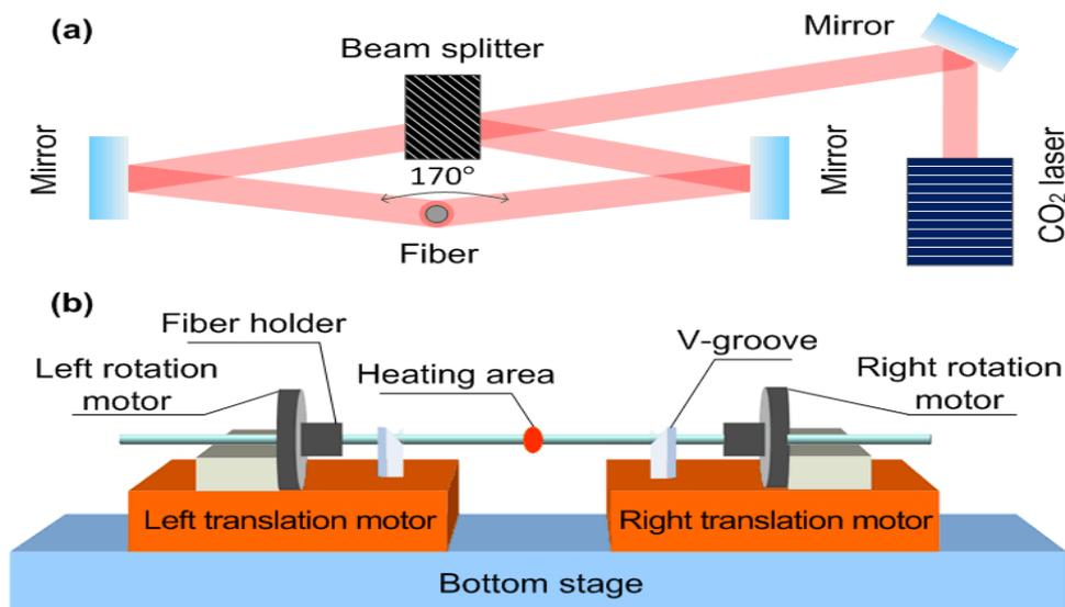
Fig. 1. (a) Optical path diagram of  $\text{CO}_2$  fusion splicer; (b) Overall diagram of  $\text{CO}_2$  fusion splicer (color online)
