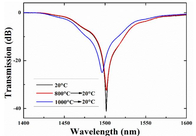
Fig. 7. Spectra of a grating with a period of 685  $\mu\text{m}$  measured after annealing from 800°C and 1000°C to 20°C (color online)
