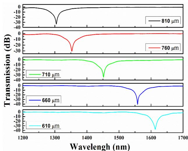
Fig.4. Spectra of gratings with periods of  $610 \mu\text{m}$ ,  $660 \mu\text{m}$ ,  $710 \mu\text{m}$ ,  $760 \mu\text{m}$  and  $810 \mu\text{m}$  (color online)
