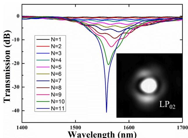
Fig. 3. Transmission spectra of the grating with a period of  $660 \mu\text{m}$  under the conditions of different number of tapering. Inset is the near-field mode field distribution of grating with an  $N = 40$  at the wavelength of  $1558 \text{ nm}$  (color online)
