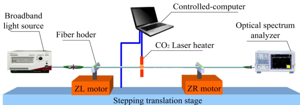
Fig. 2. Systematic diagram of fabricating MLPFGs based on microfibers (color online)
