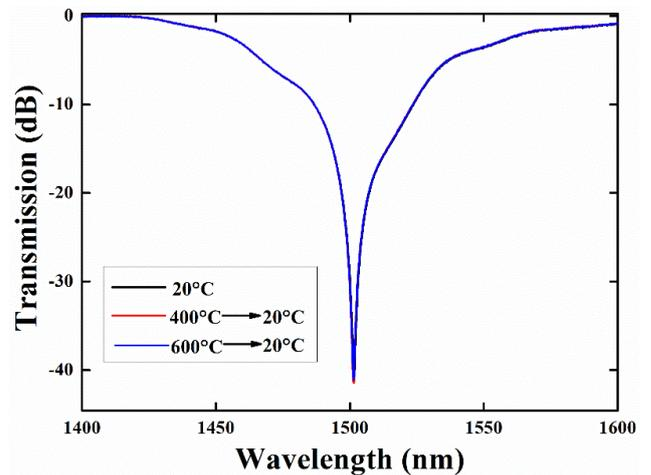
Fig. 6. Spectra of gratings with a period of 685  $\mu\text{m}$  measured after annealing from 400°C and 600°C to 20°C (color online)
