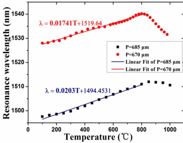
Fig. 5. Resonant wavelengths of the gratings with periods of 685  $\mu\text{m}$  and 670  $\mu\text{m}$  as a function of temperature (color online)
