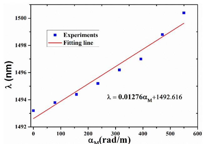
Fig. 8. Resonant wavelengths of grating as a function of the mechanical torsion rate  $\alpha_M$
