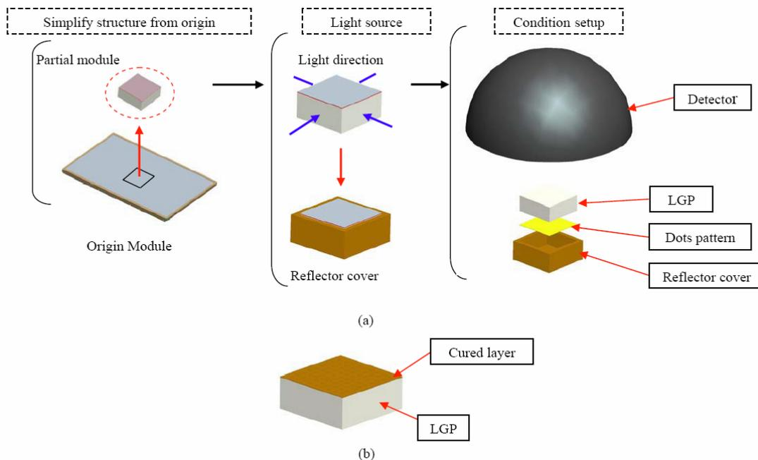
Fig. 2 (a) Model of optical simulation setup (b) The imprinting layer is attached to the LGP.
