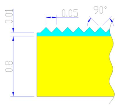
Fig. 1 Single layer of prismatic structure on the LGP, in mm.
