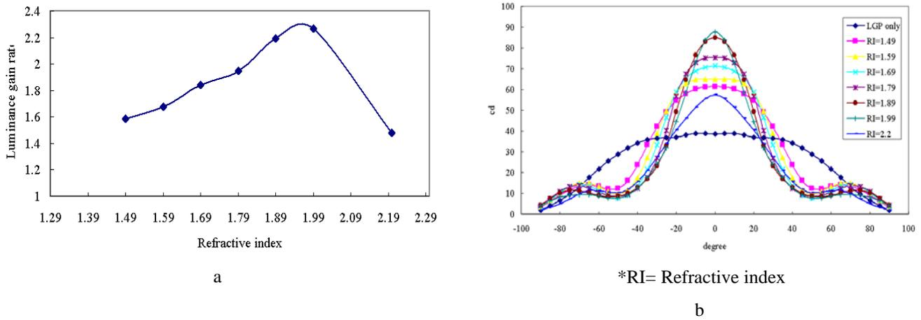
Fig. 3. (a) The gain rate distribution of LGP with single layer of prismatic structure. (b) The angular distribution of the luminous intensity.
