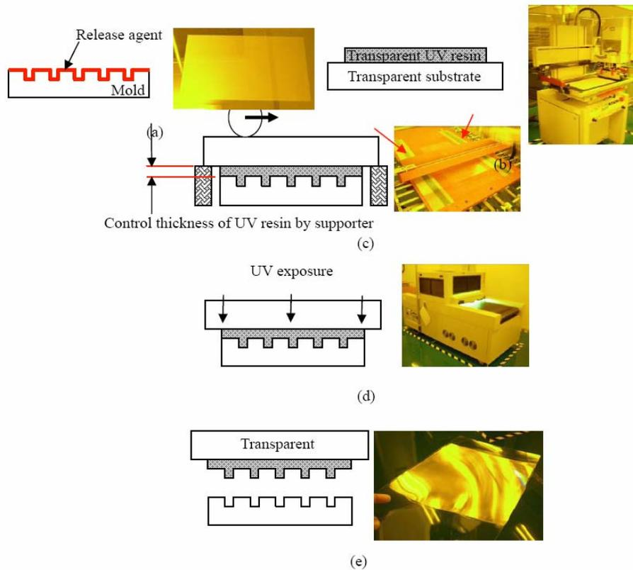
Fig. 4 Schematic diagram of the manufacturing process of the flexible mold. (a) Model of steel plate coated with a layer of release agent. (b) Substrate coated with UV resin by screen printing machine. (c) UV resin thickness controlled by support plates. (d) UV exposure using the UV light source. (e) The transparent mold released from the model.
