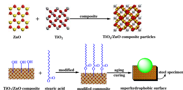
Fig. 1. Schematic illustration of superhydrophobicity coating.
