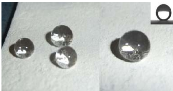
Fig. 5. Pictures of water droplets on coating.
