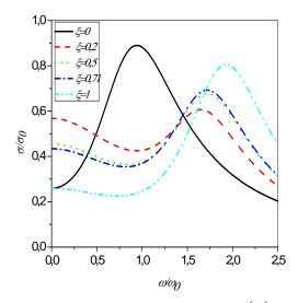
Fig. 3. Dependence of dynamic conductivity  $\sigma(\omega)$  with the frequency  $\omega$  for different values of  $\xi$ . The other parameters are  $\Gamma = 7$ , T = 300 K,  $V_I = 0.1$ eV.
