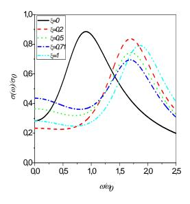
Fig. 5. Dependence of dynamic conductivity  $\sigma(\omega)$  with the frequency  $\omega$  for different values of  $\xi$ . The other parameters are  $\Gamma$ =7, T=300 K,  $V_I$  =0.1eV.
