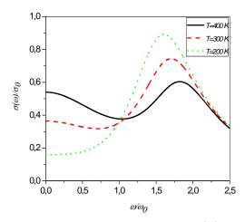
Fig. 6. Dependence of dynamic conductivity  $\sigma(\omega)$  with the frequency  $\omega$  for different values of T. The other parameters are  $\Gamma=7$ ,  $\xi=0.5$  and,  $V_1=0.1eV$ .
