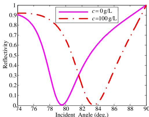
Fig. 5. SPR spectrum with different glucose concentration,
