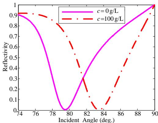
Fig. 5. SPR spectrum with different glucose concentration,  $C=0\text{g/L}$  and  $C=100\text{g/L}$  (color online)
