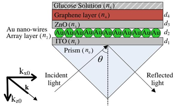
Fig. 2. Structure designed for the glucose concentration sensor (color online)
