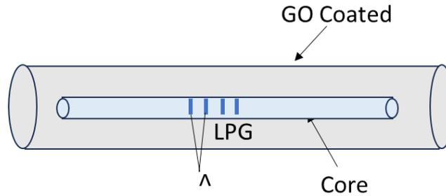
Fig. 1. The Graphene-Based LPG Fiber Sensor diagram
