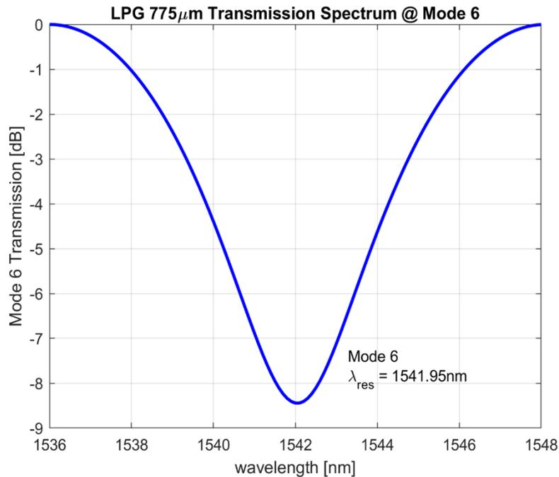
Fig. 7. Transmission spectrum of a Long Period Grating (LPG) with a period of 775  $\mu$ m at Mode 6 (colour online)
