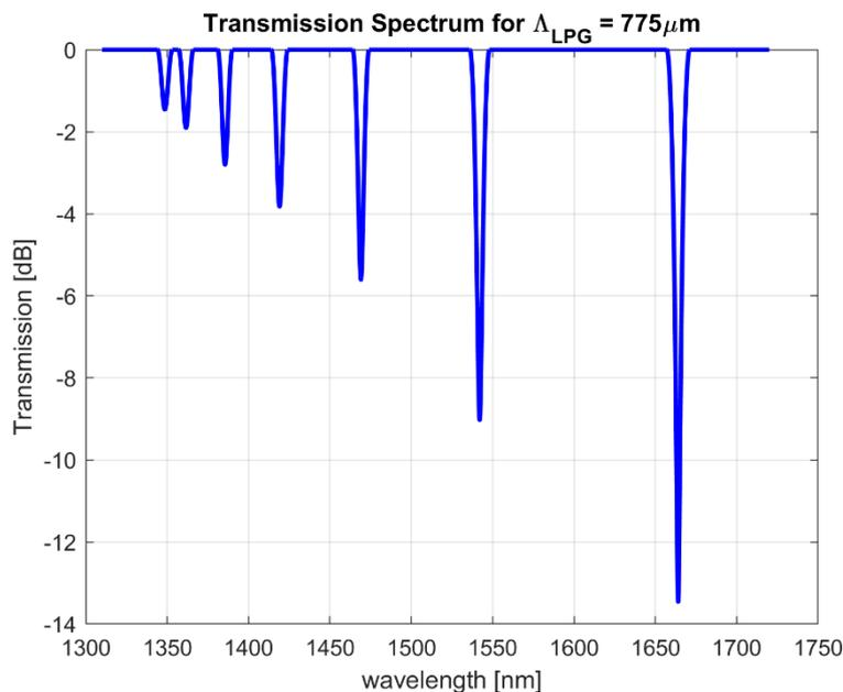
Fig 6. Transmission spectrum calculation on the basis of PMC (colour online)
