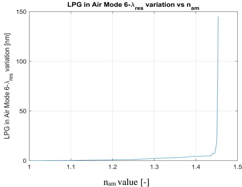
Fig. 3. Variation of the resonance wavelength of LPG in Air Mode 6 as a function of  $n_{am}$  (likely the ambient refractive index) (colour online)
