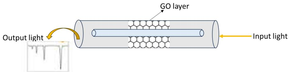
Fig. 2. Schematic view of the optical transducer based on LPG with GO (colour online)
