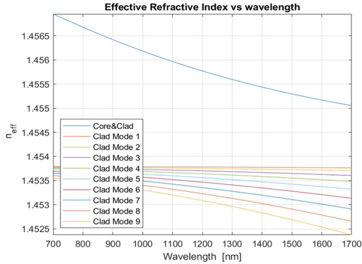
Fig. 4. Effective refractive index vs wavelength simulated for LPGFS (colour online)
