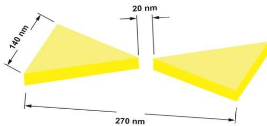
Fig.3(a). 3D schematic of the bowtie nano antenna with its structural parameters
