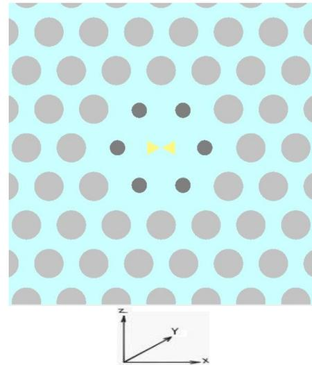
Fig. 4(a). Schematic view of the analyzed hybrid structure .The golden bowtie nano-antenna is positioned exactly at the center of the nano-cavity surface, along the x direction. The desired directions are indicated at the bottom
