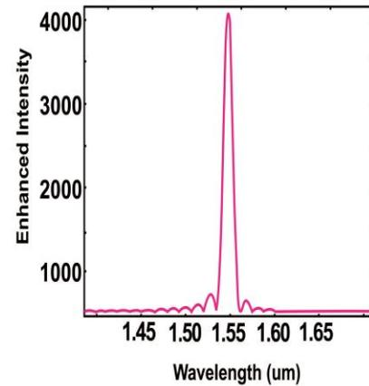
Fig. 2(a). The spectrum of the photonic crystal nano-cavity-mode
