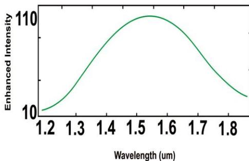
Fig. 3(b). Spectral response of the bowtie nano-antenna
