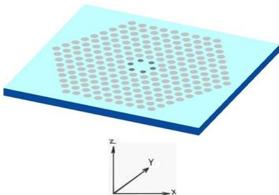
Fig. 1. 3D view of the photonic crystal cavity (The core area of the photonic crystal nano-cavity is depicted in dark gray and the cladding section is in light gray. The core and cladding parts are created in the silicon substrate, demonstrated in blue). The desired directions are indicated at the bottom
