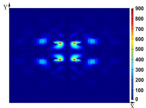
Fig. 2(c). The corresponding Y component of the electric field intensity at resonance wavelength
