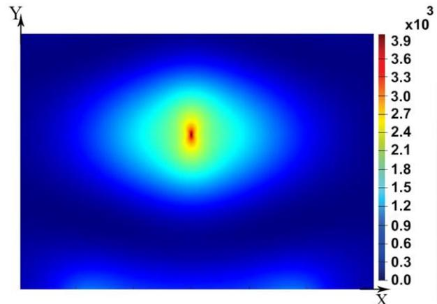
Fig. 2(b). The corresponding X component of the electric field intensity at resonance wavelength
