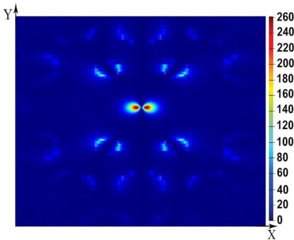
Fig. 2(d). The corresponding Z component of the electric field intensity at resonance wavelength
