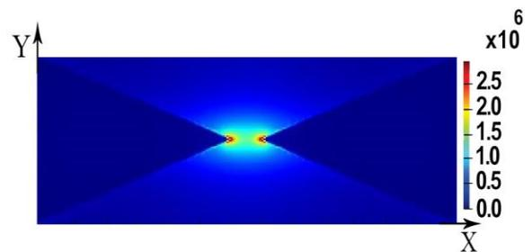
Fig. 4(c). Calculated enhancement of the electric field intensity distribution  $|E|^2$  at resonance wavelength
