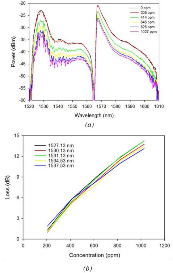
Fig. 6(a) Absorption spectra at different ammonia concentrations, (b) wavelength optical power loss at different ammonia concentration
