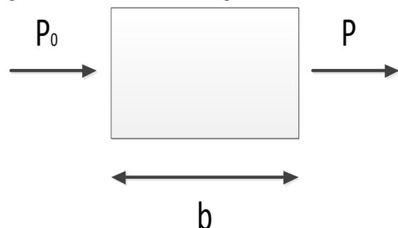
*Fig. 1 Definition of the Beer's law uses an absorbed gas inside the chamber*
