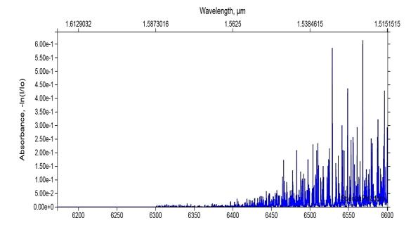
Fig. 2. The simulation spectra shows ammonia gas absorption in wavelength range of 1515- to 1612 nm. [13]
