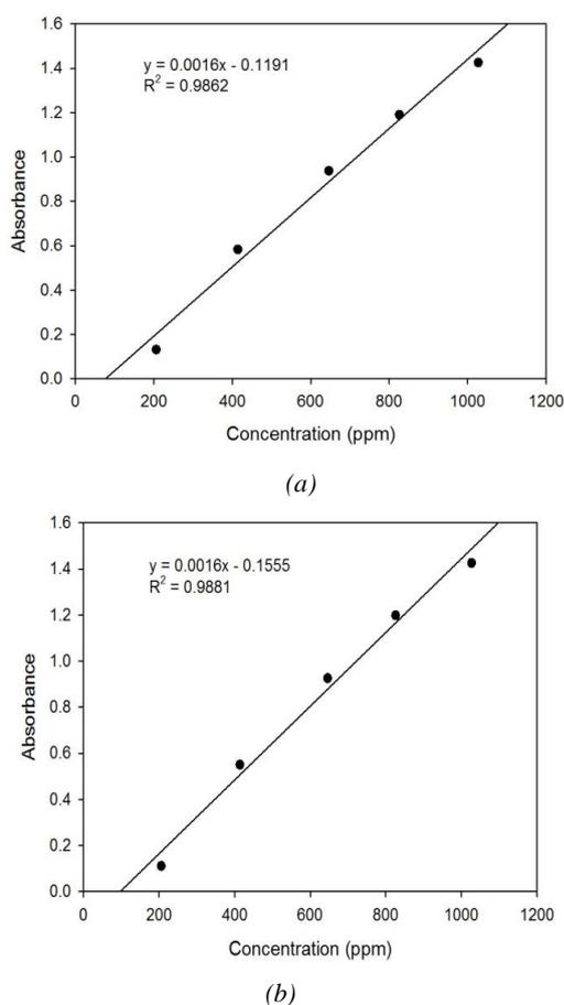
Fig. 7 Absorption at a wavelength of (a) 1527.13 nm and (b) 1531.13 at different ammonia concentrations
