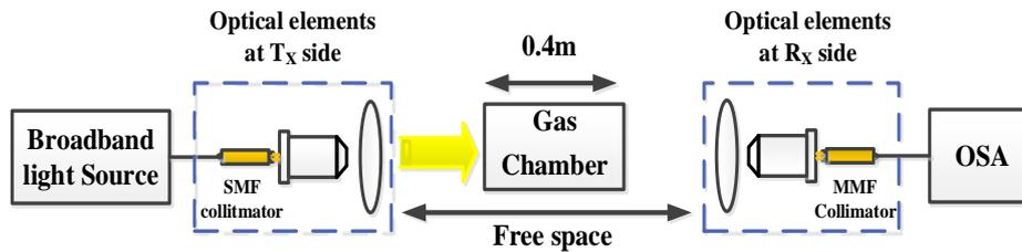
Fig. 3. Gas detection in an experimental architecture diagram (color online)
