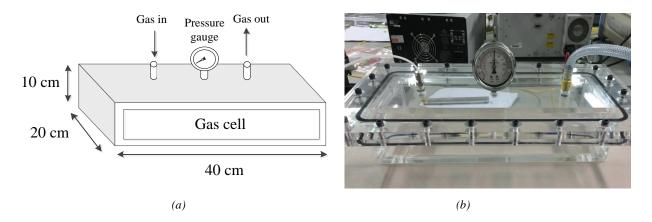
Fig. 4. (a) The designed gas chamber and (b) the customer-designed gas chamber
