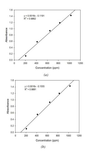
Fig. 7 Absorption at a wavelength of (a) 1527.13 nm and (b) 1531.13 at different ammonia concentrations
