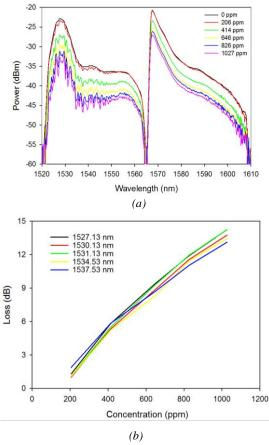
Fig. 6(a) Absorption spectra at different ammonia concentrations, (b) wavelength optical power loss at different ammonia concentration
