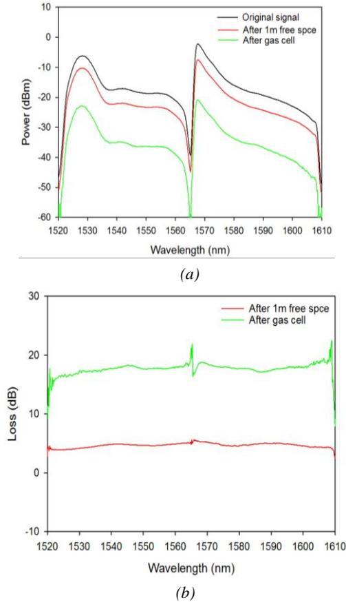
Fig. 5(a) Different spectra of a broadband source, and (b) the light power decreases spectra when compared with original light source.
