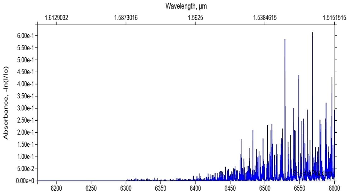
Fig. 2. The simulation spectra shows ammonia gas absorption in wavelength range of 1515- to 1612 nm. [13]
