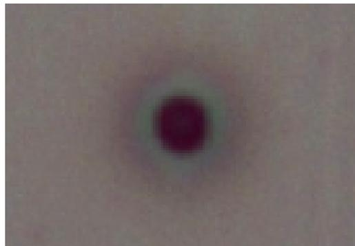
Fig. 5. Pattern of the dark spot after light exposure of amorphous  $(As_4S_3Se_3)_{0.93}Sn_{0.07}$  thin films with beam laser ( $\lambda=532.18$  nm,  $P=1$  mW).
