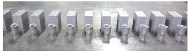
Fig. 11. Dental Ti substructure manufactured by SLM
