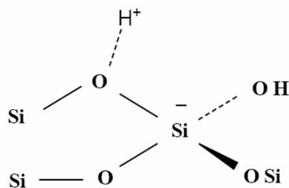
Fig. 3. Schematic presentation of the silica glass surface and silanol groups.
